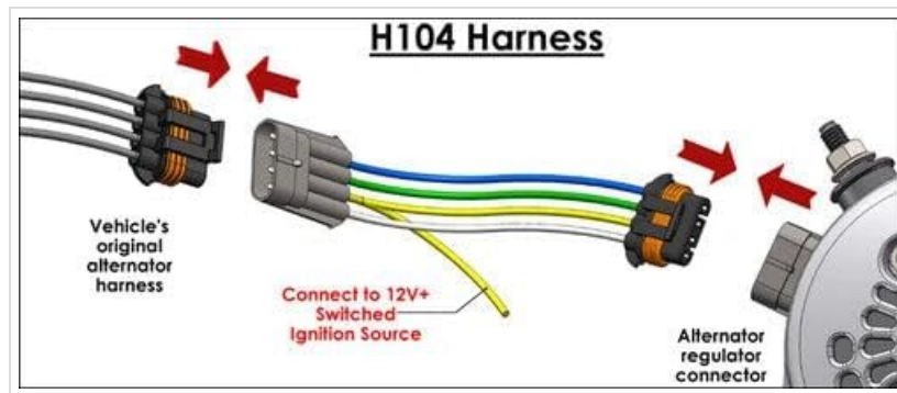
Image 4.2: Diagram illustrating the connection of the H104 harness. It shows the vehicle's original alternator harness connecting to one end of the H104, and the other end connecting to the alternator regulator connector. A yellow wire from the H104 is indicated to connect to a 12V+ switched ignition source.
