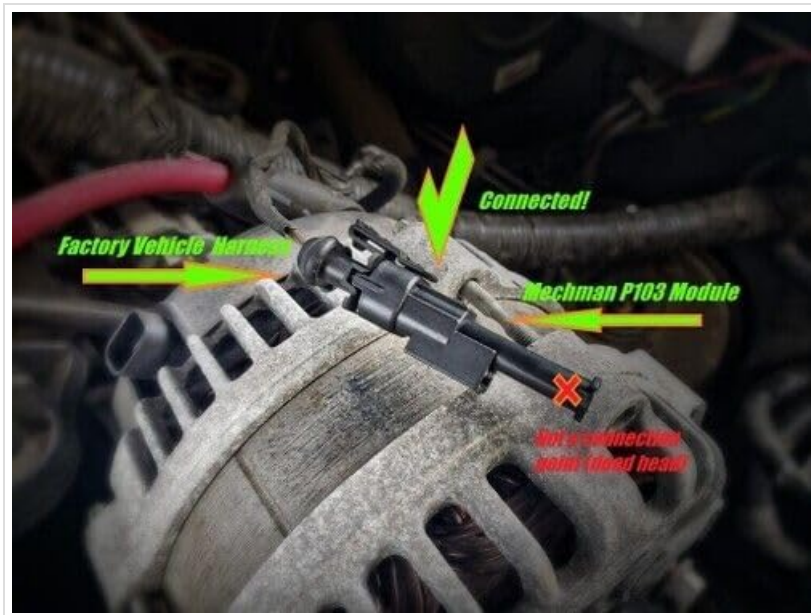
Image 4.5: Diagram showing the Mechman P103 Module connected between the factory vehicle harness and the alternator. A green checkmark indicates a correct connection, while a red 'X' indicates an incorrect connection point on the alternator's threaded head.
