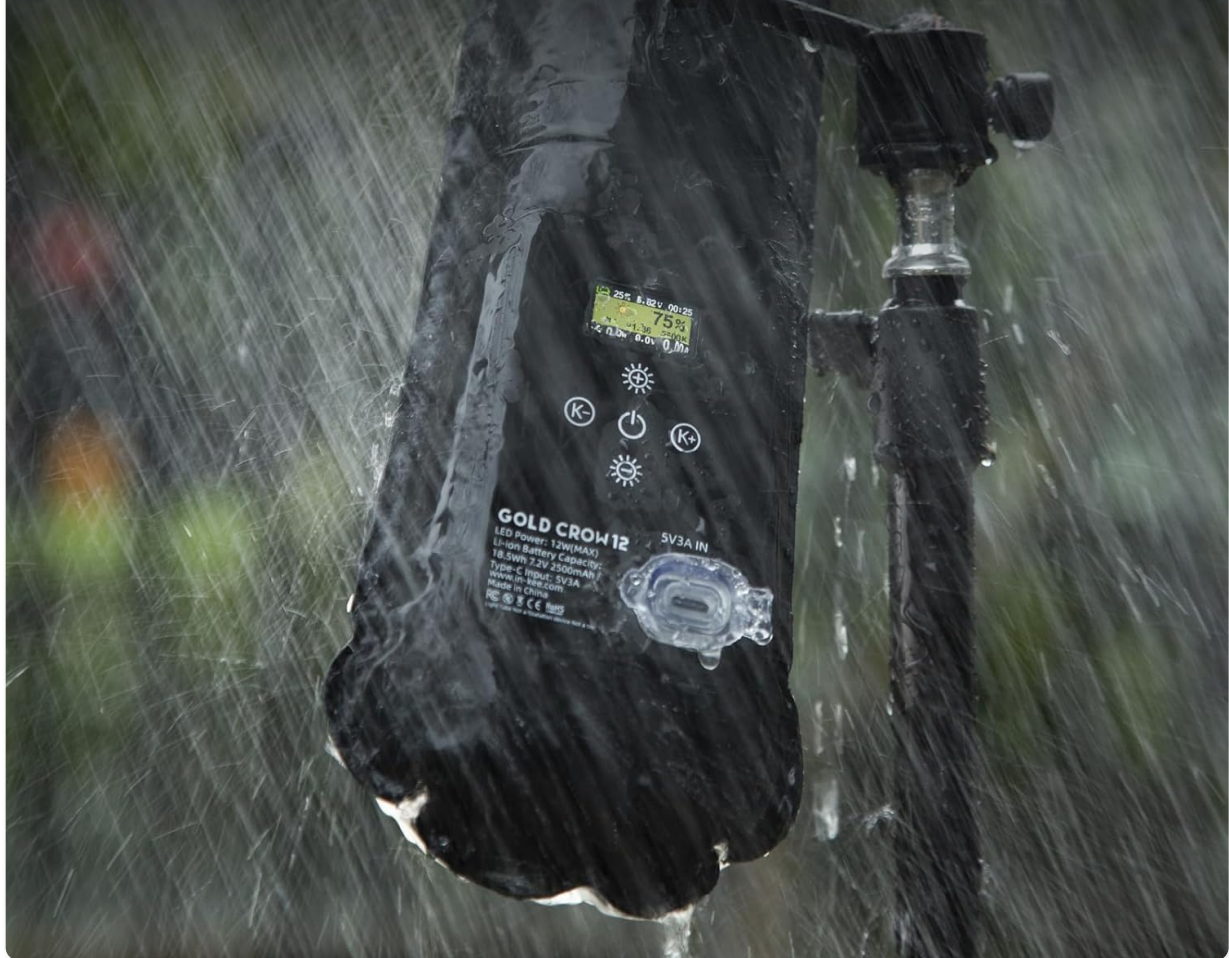
Image 5.1: The GC12 light operating under simulated rain conditions, illustrating its IP66 protection level.
