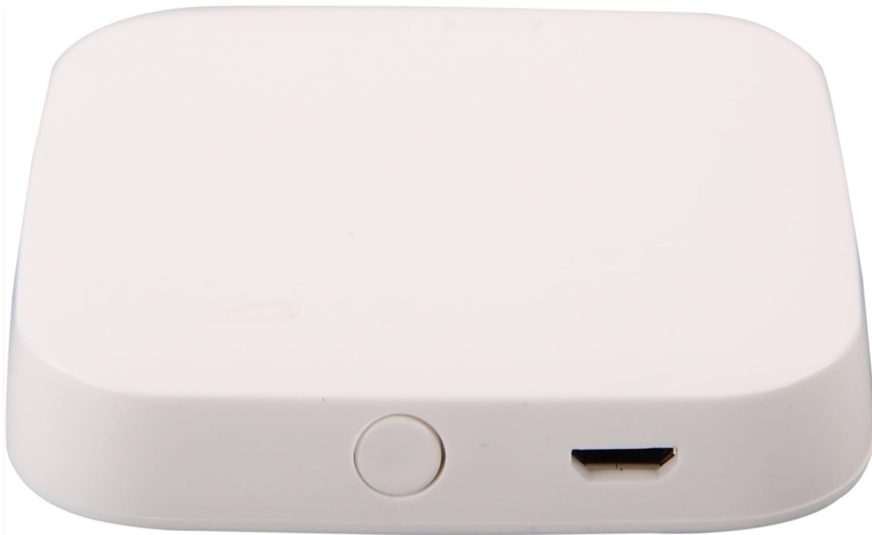
Figure 2.2: Side view of the gateway with micro-USB port.
