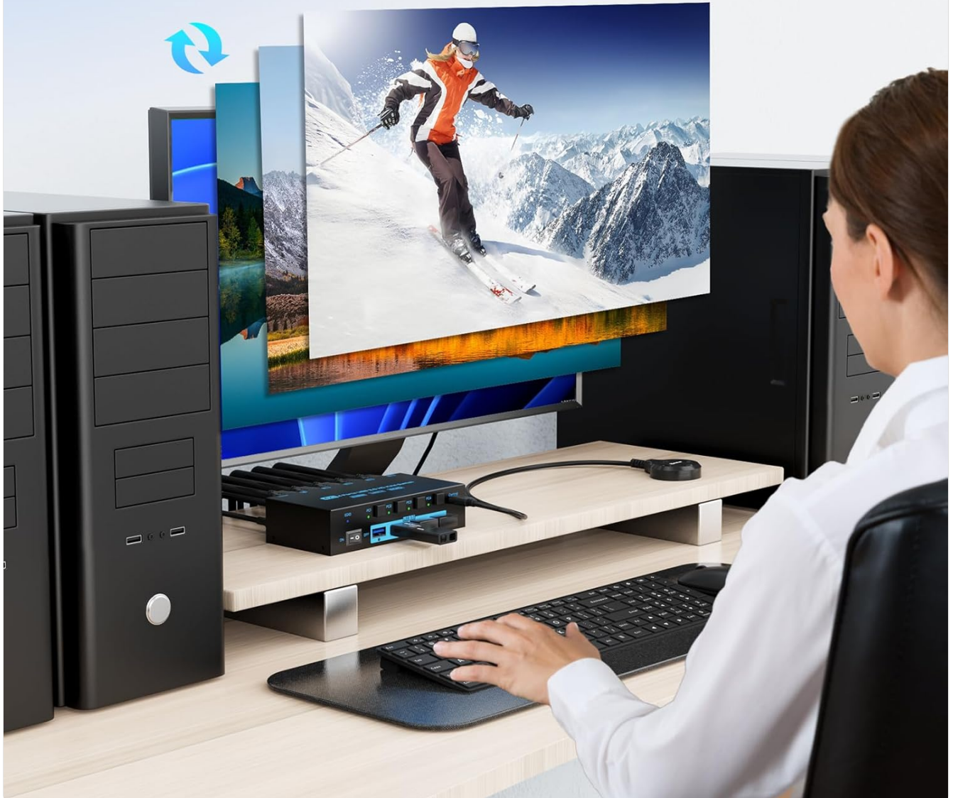
Figure 3.2: Example setup showing 4 PCs sharing 1 monitor and 4 USB 3.0 devices.
