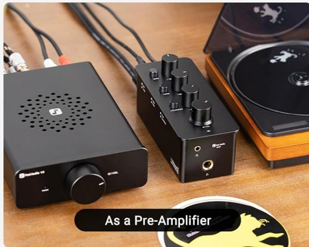
Image 4.4: SK01 demonstrating its use as a headphone amp, pre-amplifier, and equalizer.
