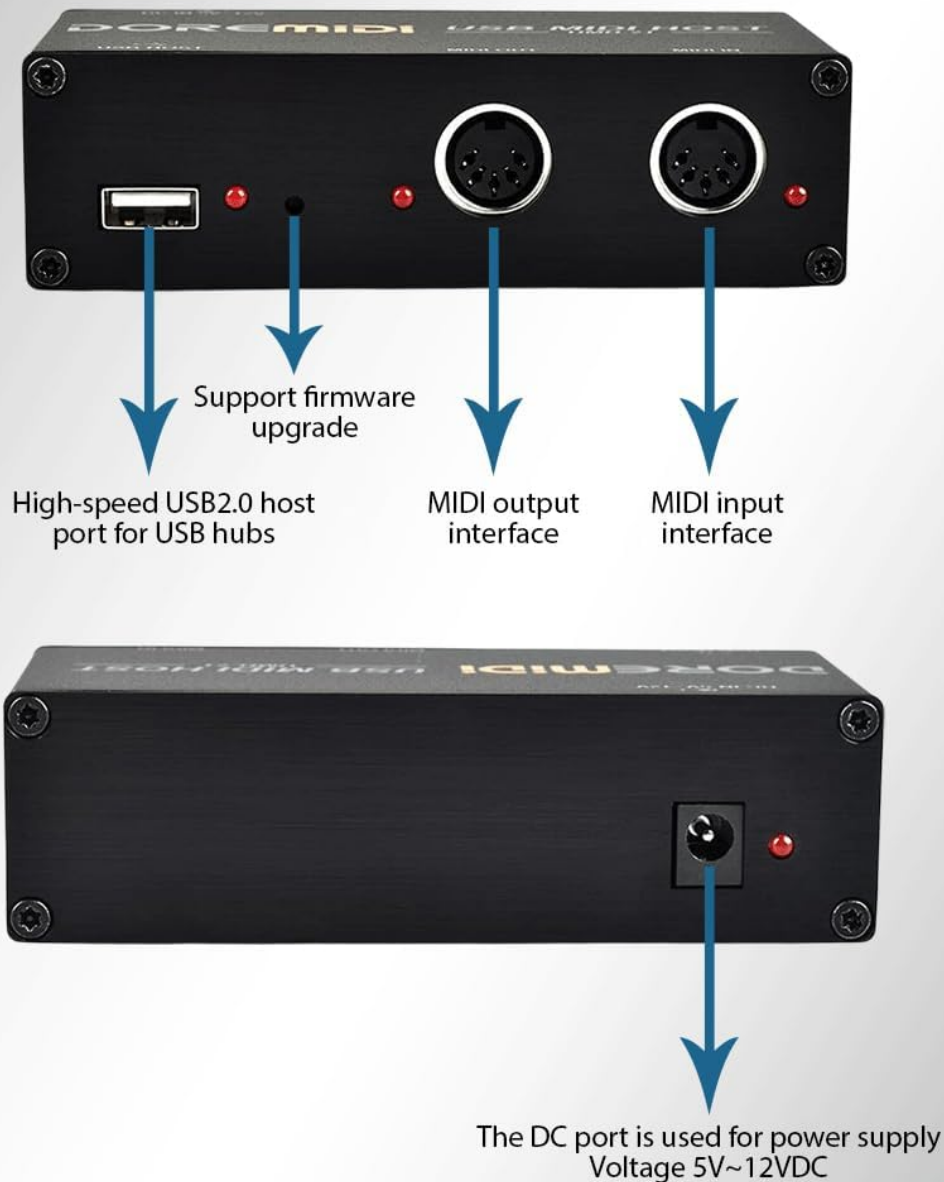
Figure 3.2: Port Diagram. This diagram provides a clear overview of the summina UMH-21's ports. The front panel includes a high-speed USB 2.0 host port for USB hubs, a MIDI output interface, and a MIDI input interface. The rear panel shows the DC port for power supply, accepting 5V-12V DC.
