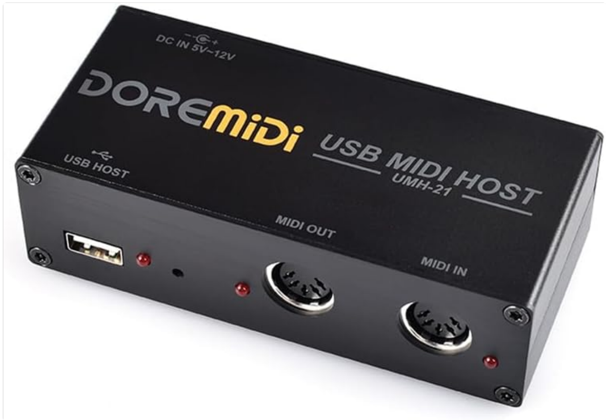
Figure 3.1: Front View of UMH-21. This image shows the front panel of the summina DOREMiDi USB MIDI Host UMH-21. It features a USB HOST port, MIDI OUT, and MIDI IN ports, along with indicator lights. The top panel indicates 'DC IN 5V-12V'.
