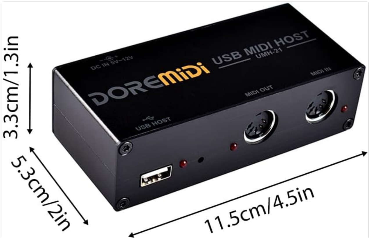
Figure 8.1: Product Dimensions. This image displays the physical dimensions of the summina UMH-21. The device measures 11.5 cm (4.5 inches) in length, 5.3 cm (2 inches) in width, and 3.3 cm (1.3 inches) in height.
