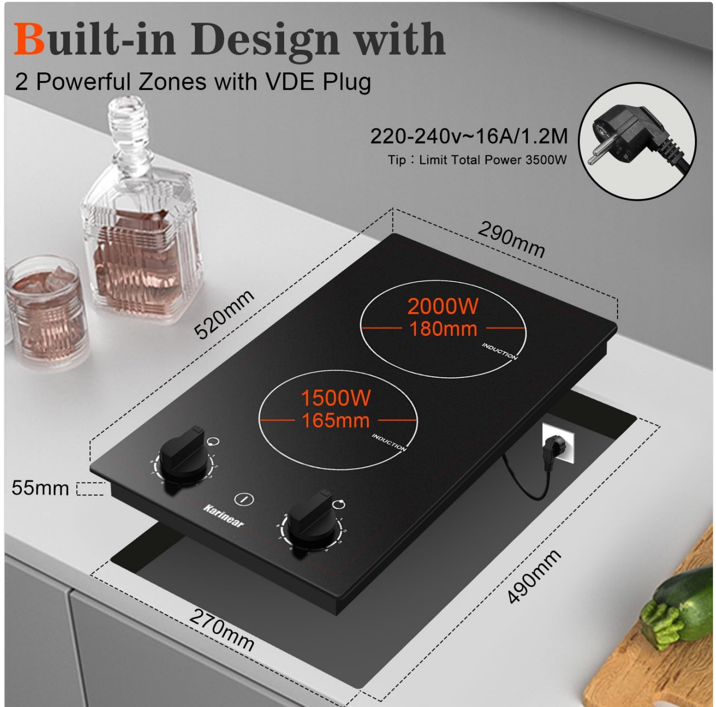
Figure 3.1: Detailed dimensions of the cooktop (520mm x 290mm x 55mm) and the recommended cut-out size (490mm x 270mm) for built-in installation. Also shows power specifications (220-240V~16A/1.2M, Total Power 3500W).
