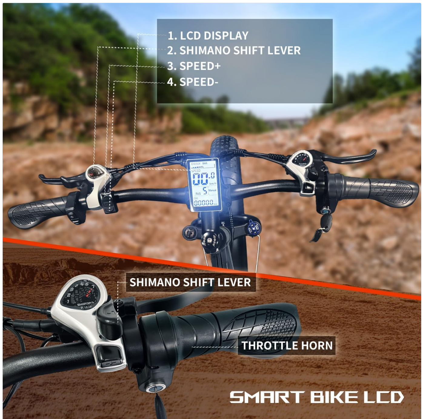
Figure 4.4: Handlebar controls including the LCD display, Shimano shift lever, and throttle.
