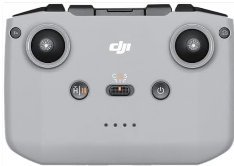
Figure 1: Front view of the Opus RC-N2 Remote Controller. This image displays the two primary control sticks, the power button, the flight mode switch, and the function (Fn) button. Battery indicator lights are visible at the bottom.
