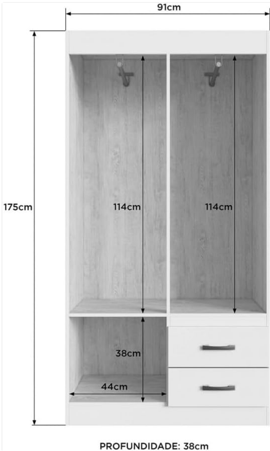
Image 8.1: Detailed diagram showing the dimensions of the Doripel Cordova Single Wardrobe, including overall height, width, depth, and internal compartment measurements.
