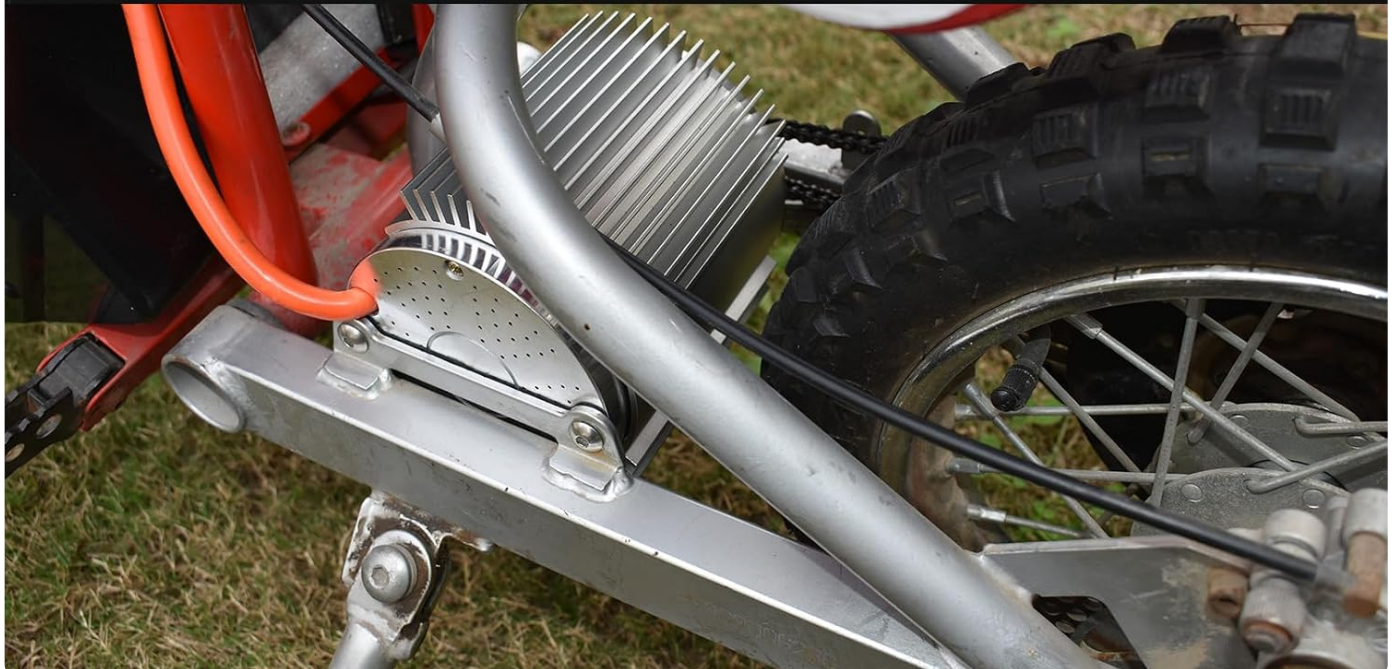
Figure 6: Motor installation hole for M6 screws (95mm diameter).
