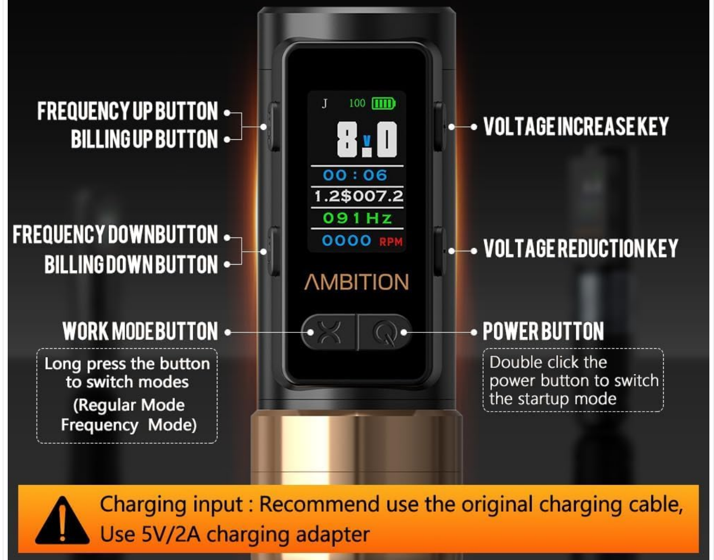
Image illustrating the multi-functional display and charging input recommendation (5V/2A adapter).
