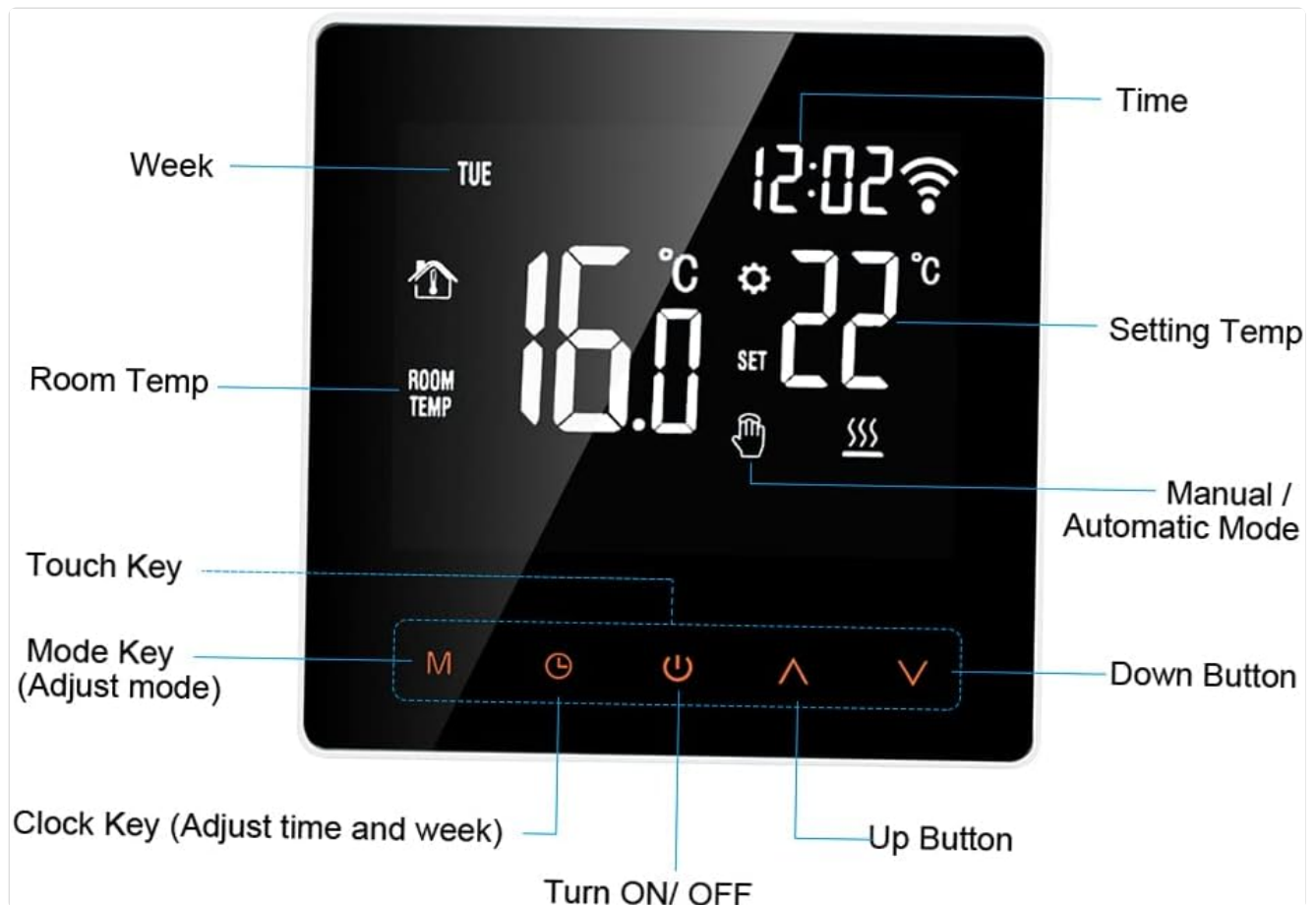
Figure 2: Labeled diagram of the thermostat's display and touch keys, indicating Time, Week, Room Temp, Setting Temp, Touch Key, Mode Key, Clock Key, Turn ON/OFF, Up Button, and Down Button.
