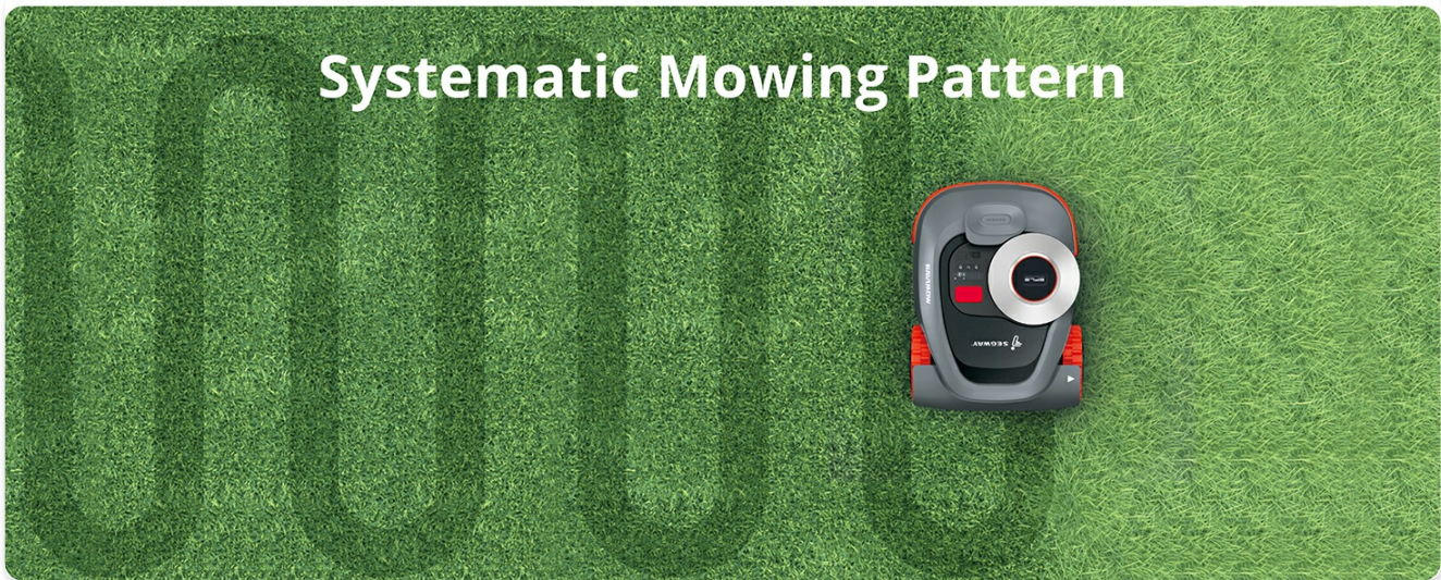
Figure 5.1: The Navimow's systematic mowing pattern ensures thorough and efficient coverage of the lawn, resulting in a uniform cut.
