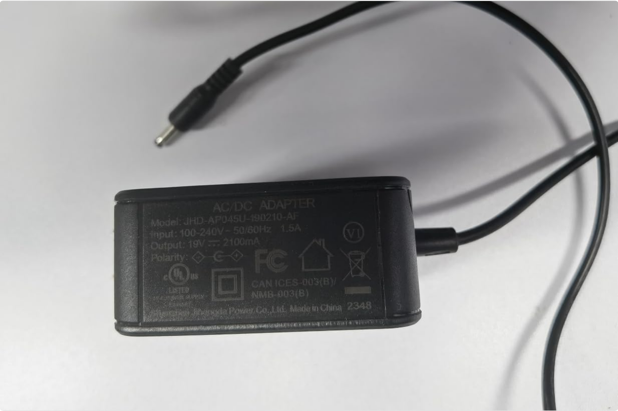
Image 2: Bottom view of the ACEMAGIC AX16 Charger and Adapter. This image displays the product label with detailed electrical specifications and compliance markings.
