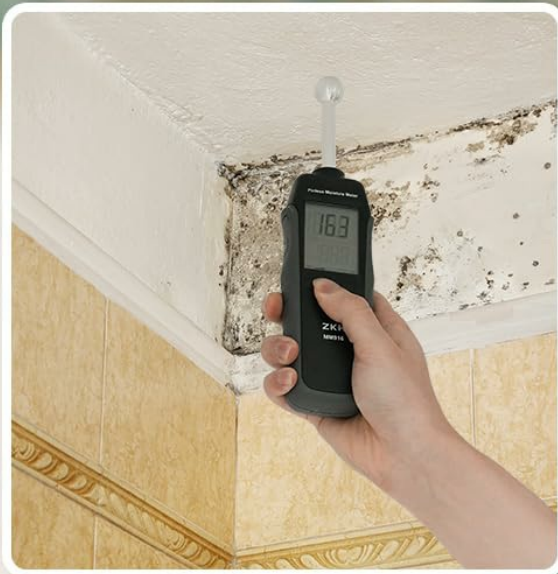
Image 5.4: Examples of the ZKH Pinless Moisture Meter in use across different materials and scenarios, including wood, wooden floors, concrete walls, ceramic tiles, ceiling tiles, and caravan interiors.
