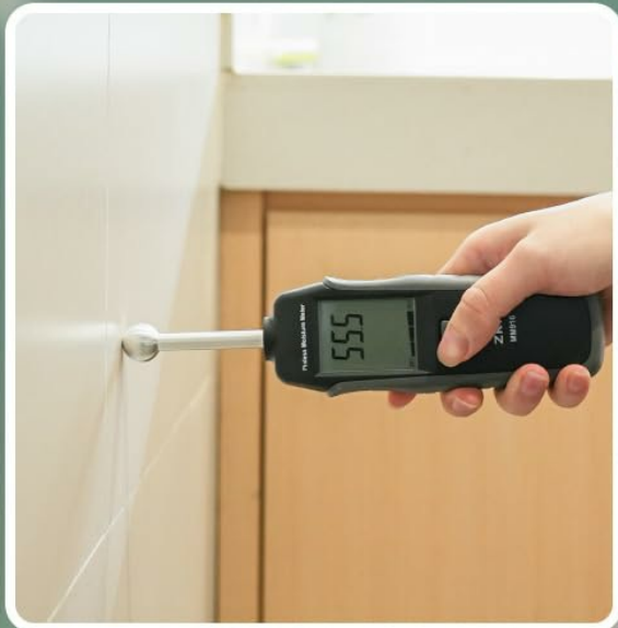
Image 5.4: Examples of the ZKH Pinless Moisture Meter in use across different materials and scenarios, including wood, wooden floors, concrete walls, ceramic tiles, ceiling tiles, and caravan interiors.
