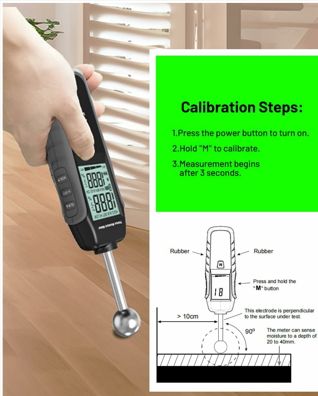
Image 4.1: Illustration of the calibration process for the ZKH Pinless Moisture Meter. A hand holds the meter, demonstrating the correct position for calibration and measurement.
