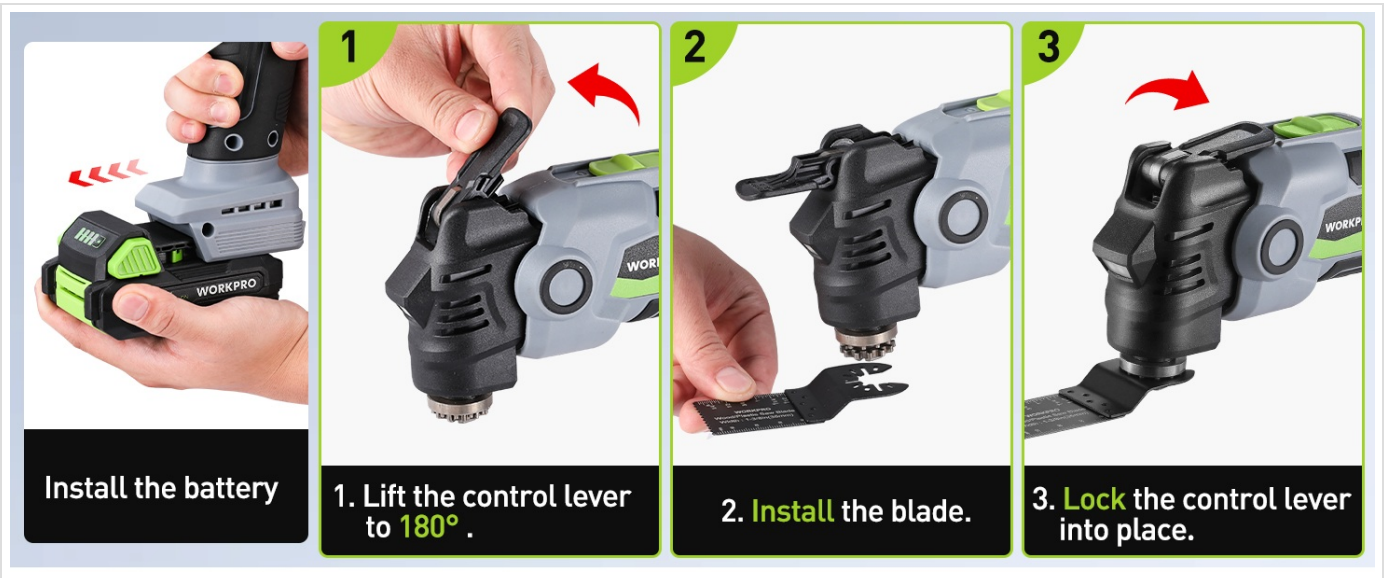
Figure 3.1: Visual guide for battery installation and the 3-step accessory changing process: 1. Install the battery. 2. Lift the control lever to 180 degrees. 3. Install the blade and lock the control lever into place.
