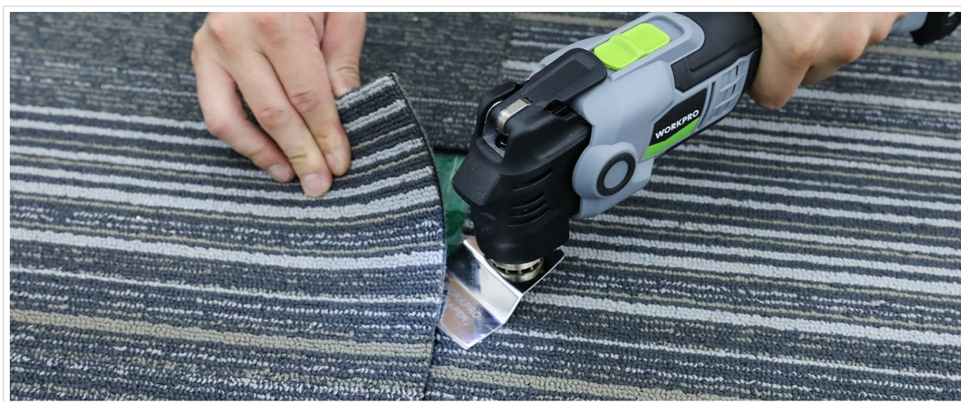
Figure 4.4: The oscillating tool with a scraper attachment, effectively removing material from a surface.
