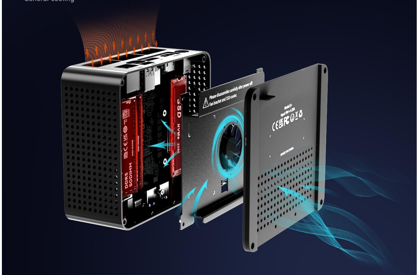
Internal view illustrating the heat dissipation system.
