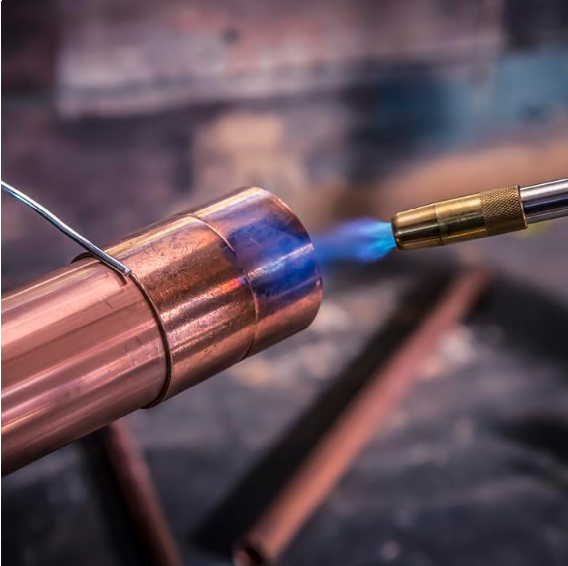
Image: The Bernzomatic TS4000 torch in action, heating a copper pipe for soldering, demonstrating the precise and powerful swirl flame.
