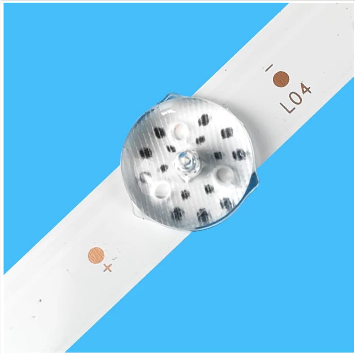
Figure 4.2: Close-up view of an individual LED and its lens on the backlight strip, demonstrating the light source.
