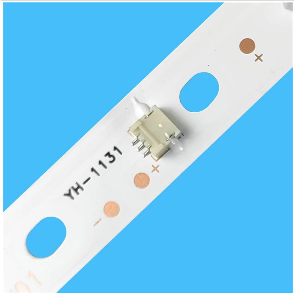
Figure 4.1: Detail of the power connector on the LED backlight strip, showing the connection points.
