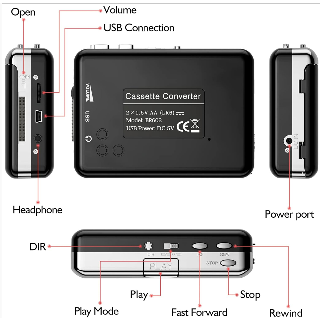
Figure 3.1: Labeled diagram of the Mersoco BR602S Cassette Player, showing controls such as Volume, USB Connection, Headphone Jack, DIR button, Play Mode, Play, Fast Forward, Rewind, Stop, and Power Port.
