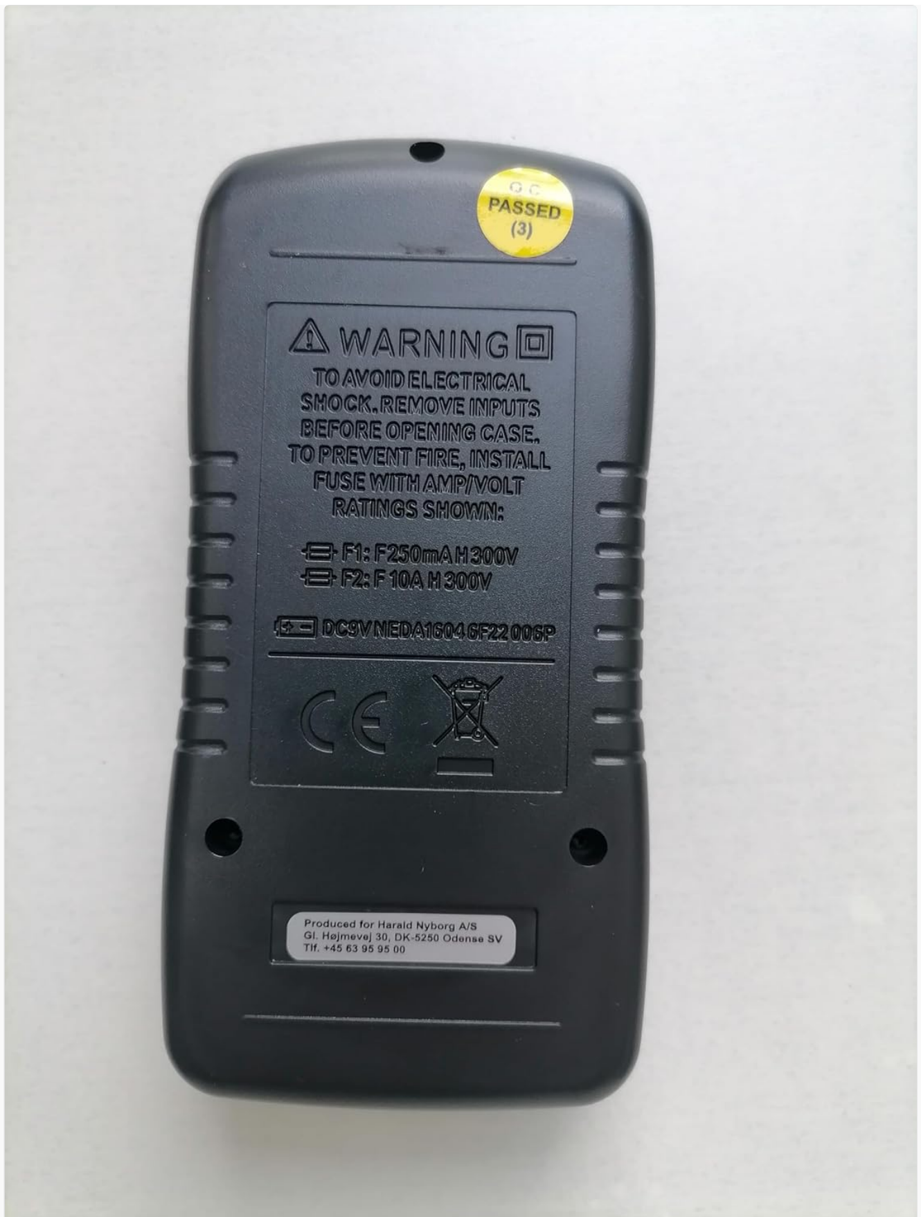
Figure 2.1: Back of the Mastech MAS830L Multimeter, showing important safety warnings and fuse specifications.
