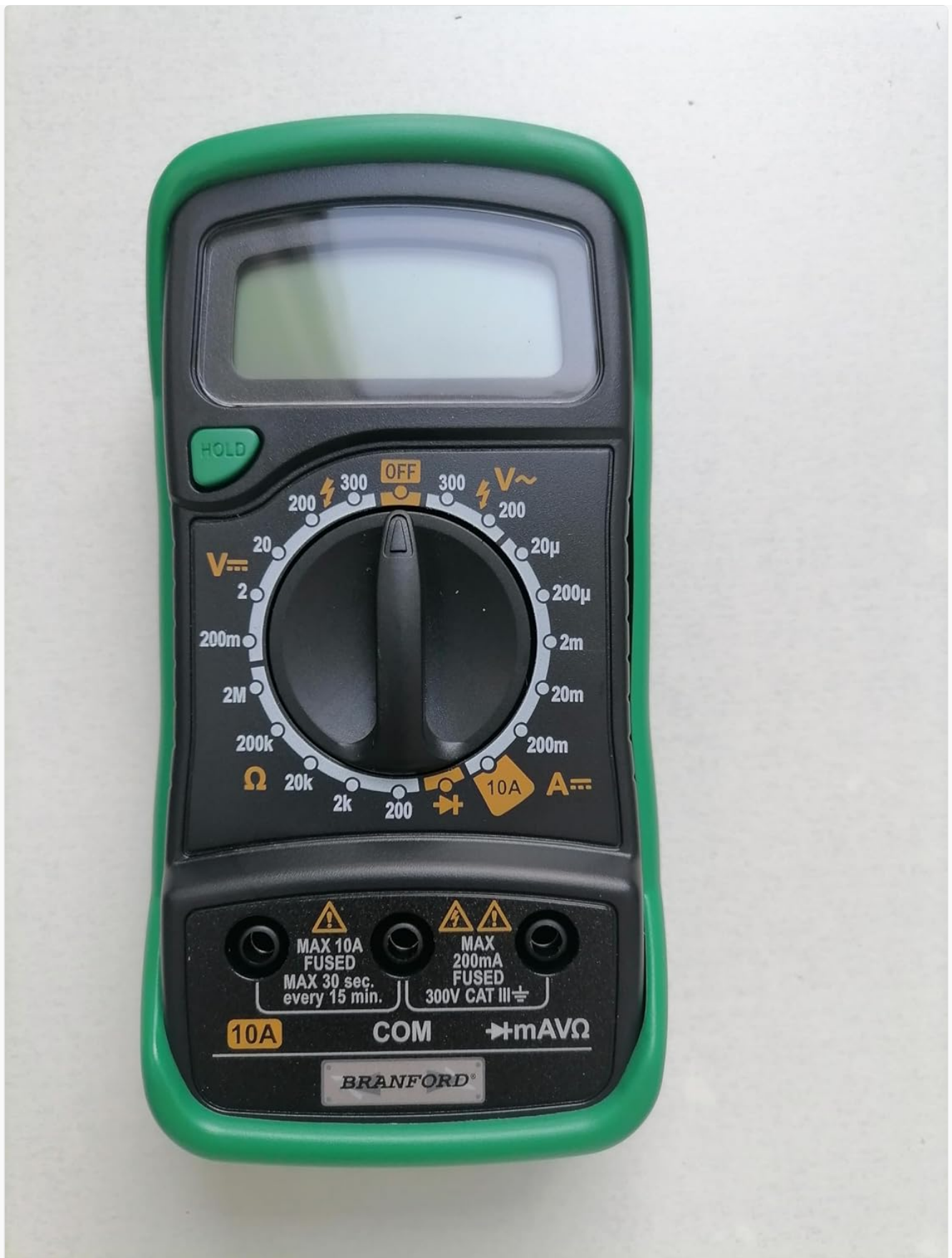
Figure 5.1: Close-up view of the Mastech MAS830L's function dial and input jacks, illustrating the various measurement settings.
