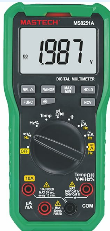
Figure 4.1: Front view of the Mastech MS8251A Digital Multimeter, showing the LCD display, function buttons, rotary switch, and input jacks. This image provides a clear visual reference for identifying the various parts of the device.
