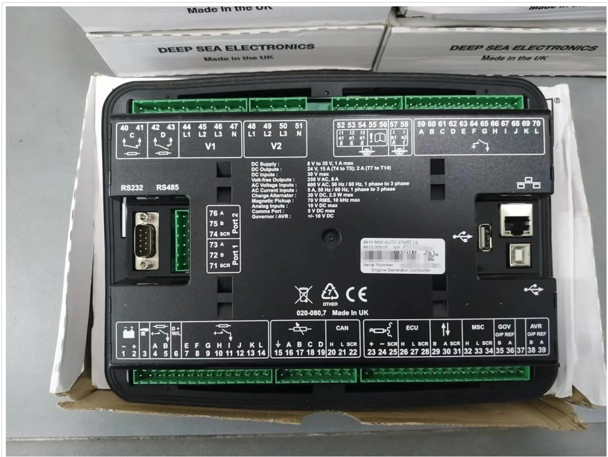
Figure 4.1: Rear view of the DSE8610MKII controller with terminal connections. This image shows the rear panel of the DSE8610 controller, detailing the various terminal blocks for electrical connections, including DC supply, AC inputs, outputs, RS232, RS485, CAN, ECU, MSC, GOV, and AVR. Key electrical specifications and certifications are also visible on the label.
