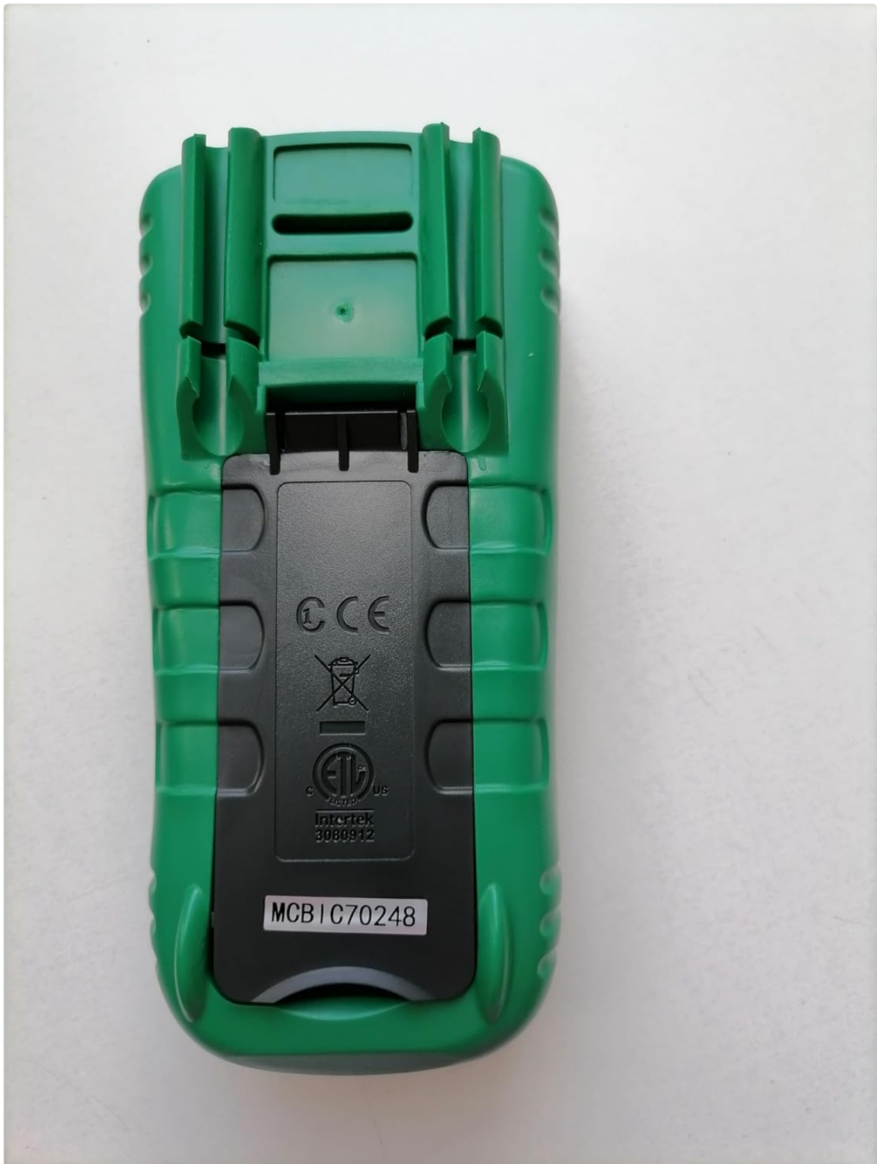
Rear view of the Mastech MS8360F multimeter, indicating the location of the battery compartment.
