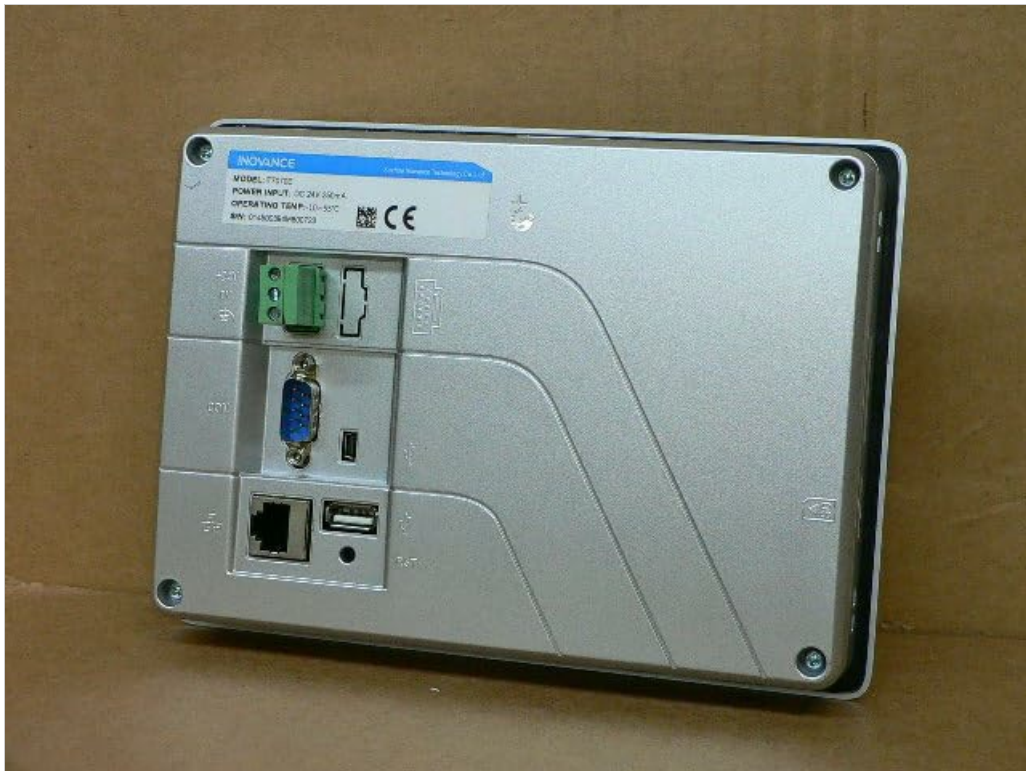
Figure 3.2: Rear view of the IT7070E module, displaying connection ports including a green terminal block, a D-sub connector, an Ethernet port, and USB ports.
