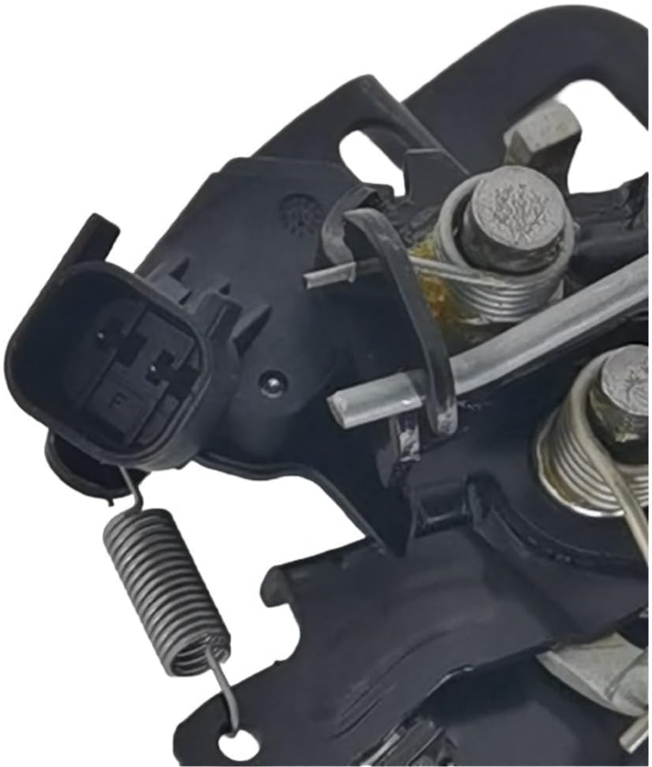
Figure 2.2: Detailed view of the electrical connector on the hood lock assembly, which may need to be connected during installation.
