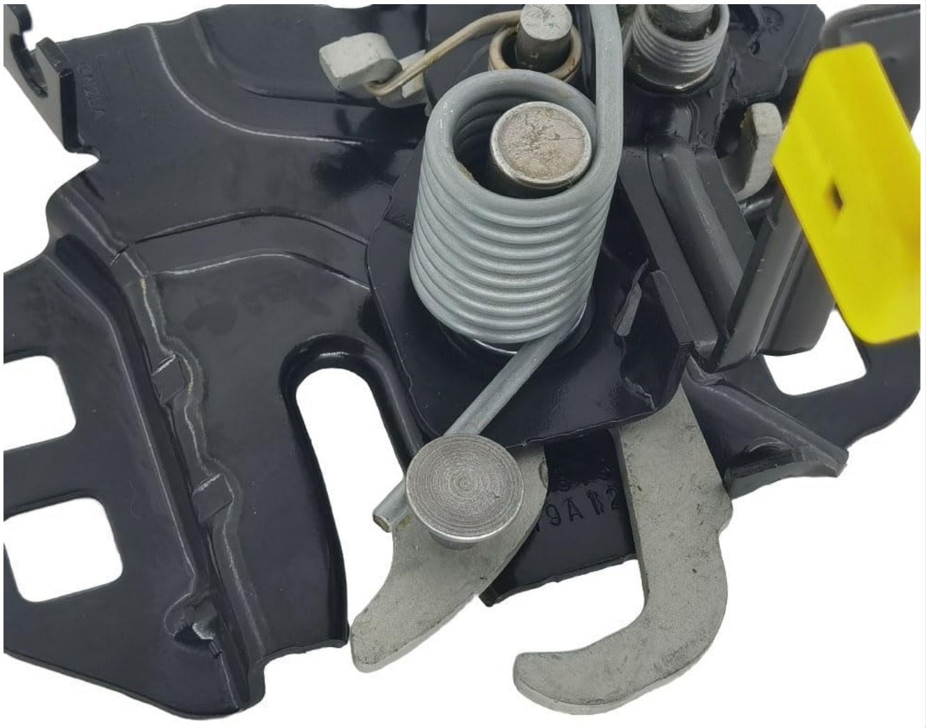
Figure 5.1: Angled view of the hood lock assembly, useful for identifying potential points of misalignment or damage during troubleshooting.
