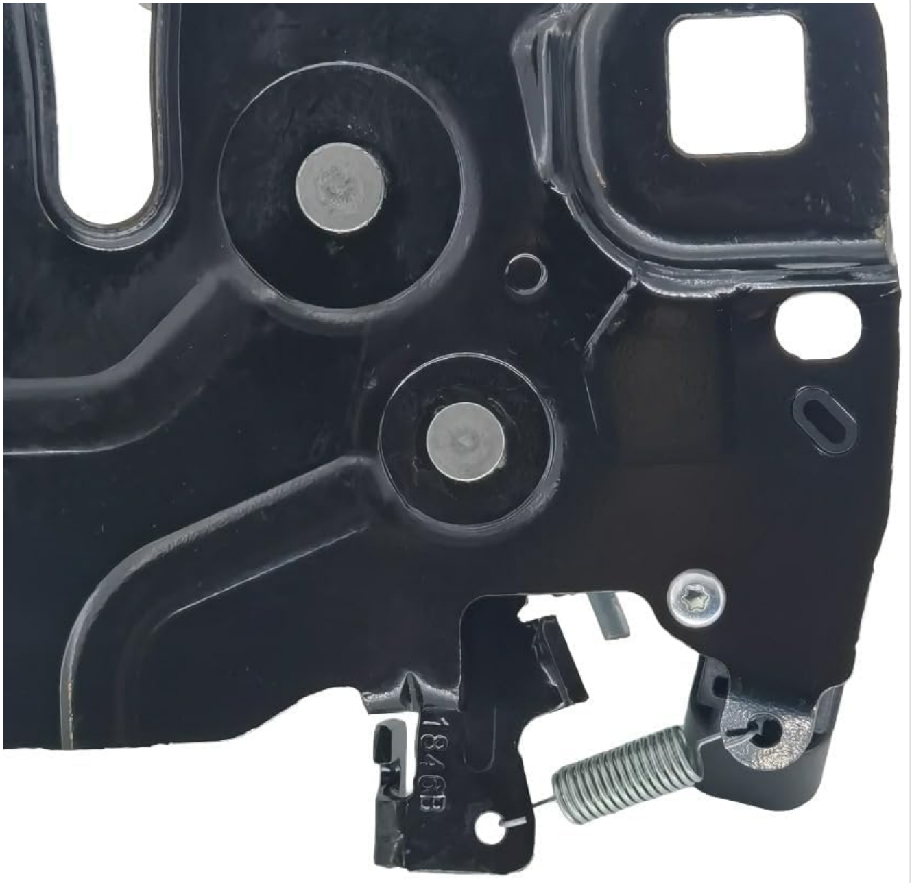
Figure 4.1: Close-up view of the spring and lever mechanism, illustrating areas that may benefit from periodic lubrication.
