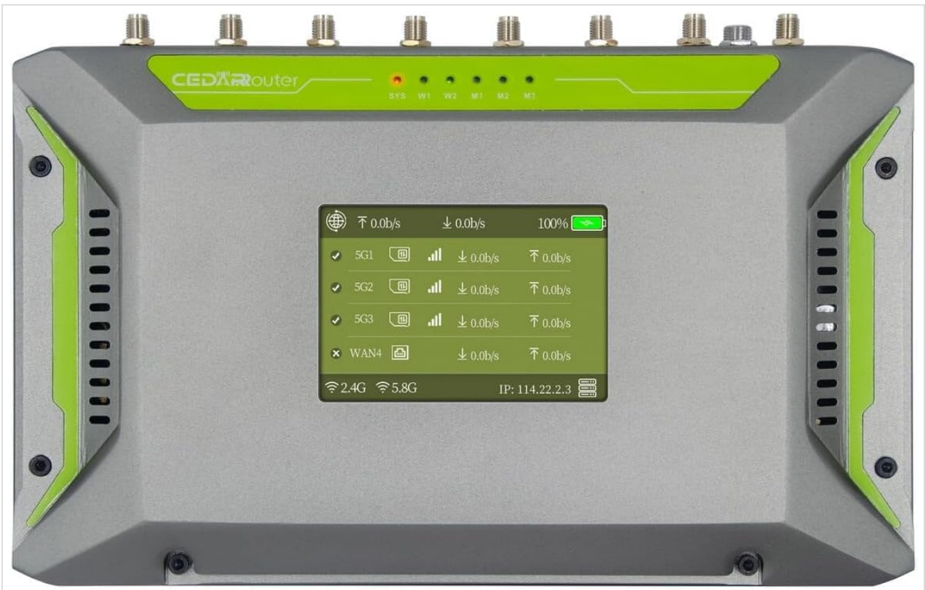
Figure 4.5: Top view showing the LCD display and status indicators.
