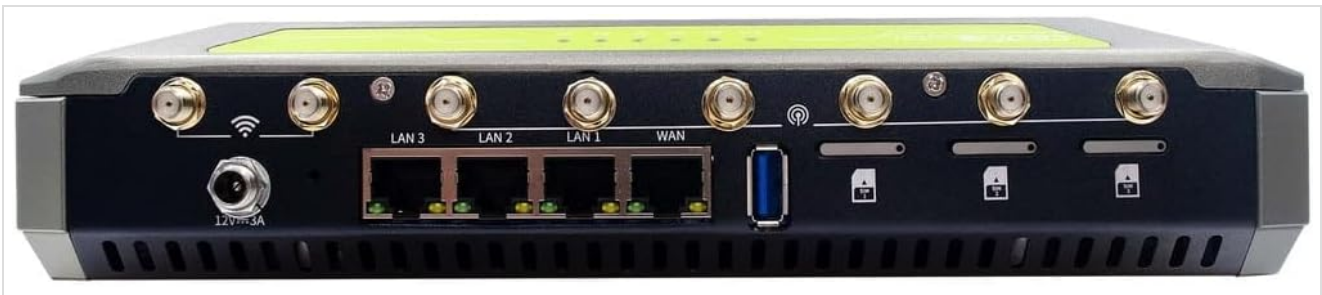
Figure 4.3: Detailed view of the rear panel, including SIM card slots.
