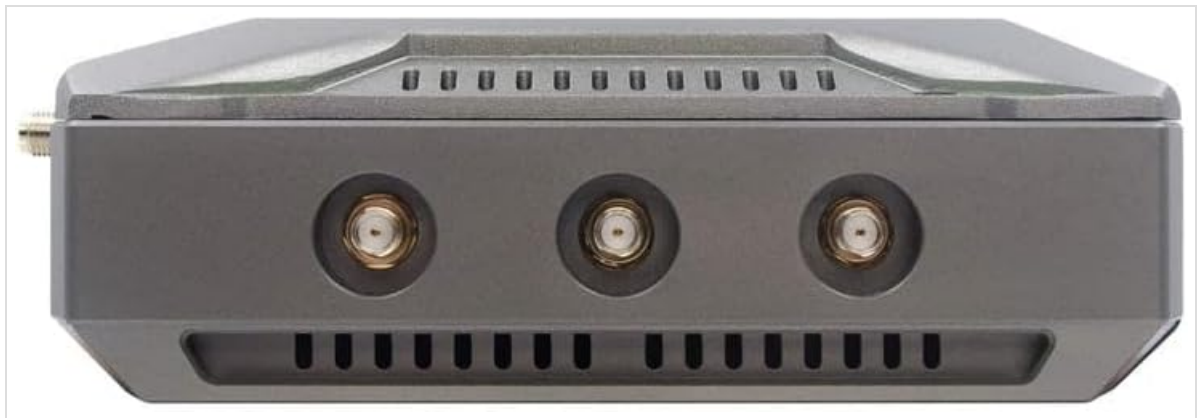
Figure 4.2: Side view showing additional antenna connectors.
