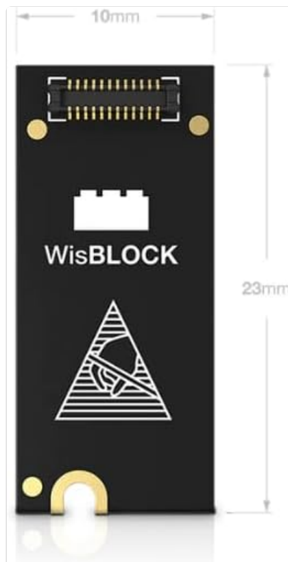
Figure 2.3: The RAK12500 module with its dimensions indicated, measuring 10 mm x 23 mm.
