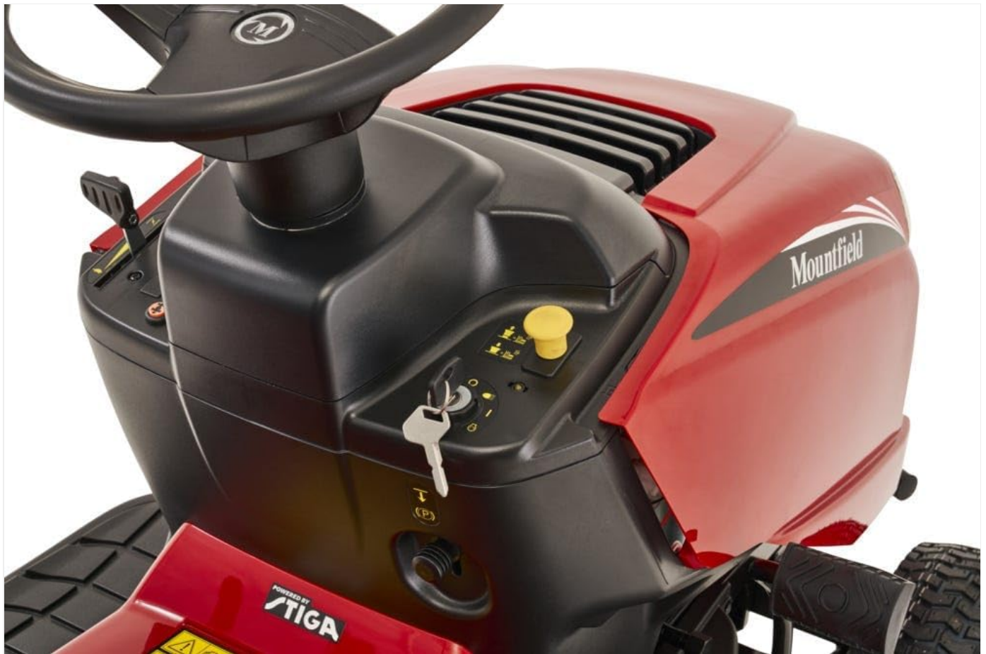
Figure 2: Driver's console showing ignition key and control layout.
