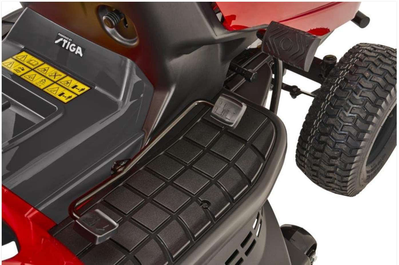
Figure 4: Foot pedal area for controlling the hydrostatic transmission.
