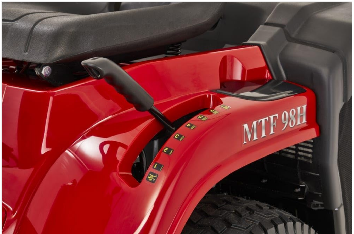
Figure 5: Cutting height adjustment lever with 7 positions (25-80 mm).
