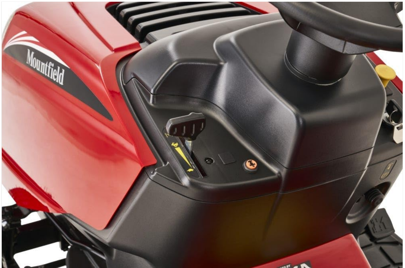
Figure 3: Detailed view of the ignition switch and choke lever.
