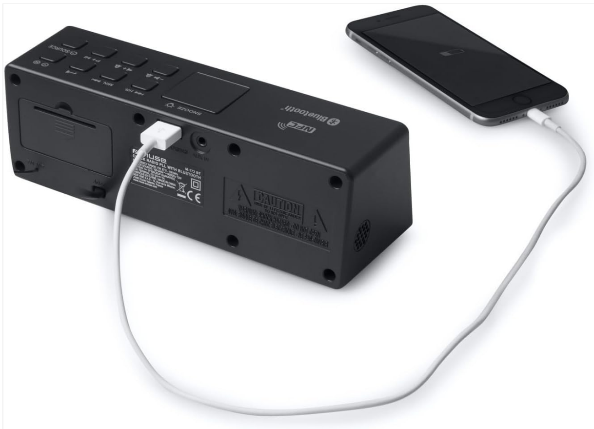
Image: Rear view of the Bmi Muse M-172-BT, detailing the connection ports.
