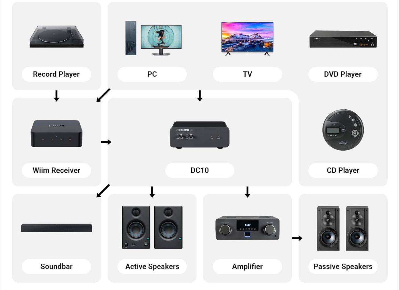
Figure 4: Connectivity scenarios for the DC10 DAC with various audio systems.
