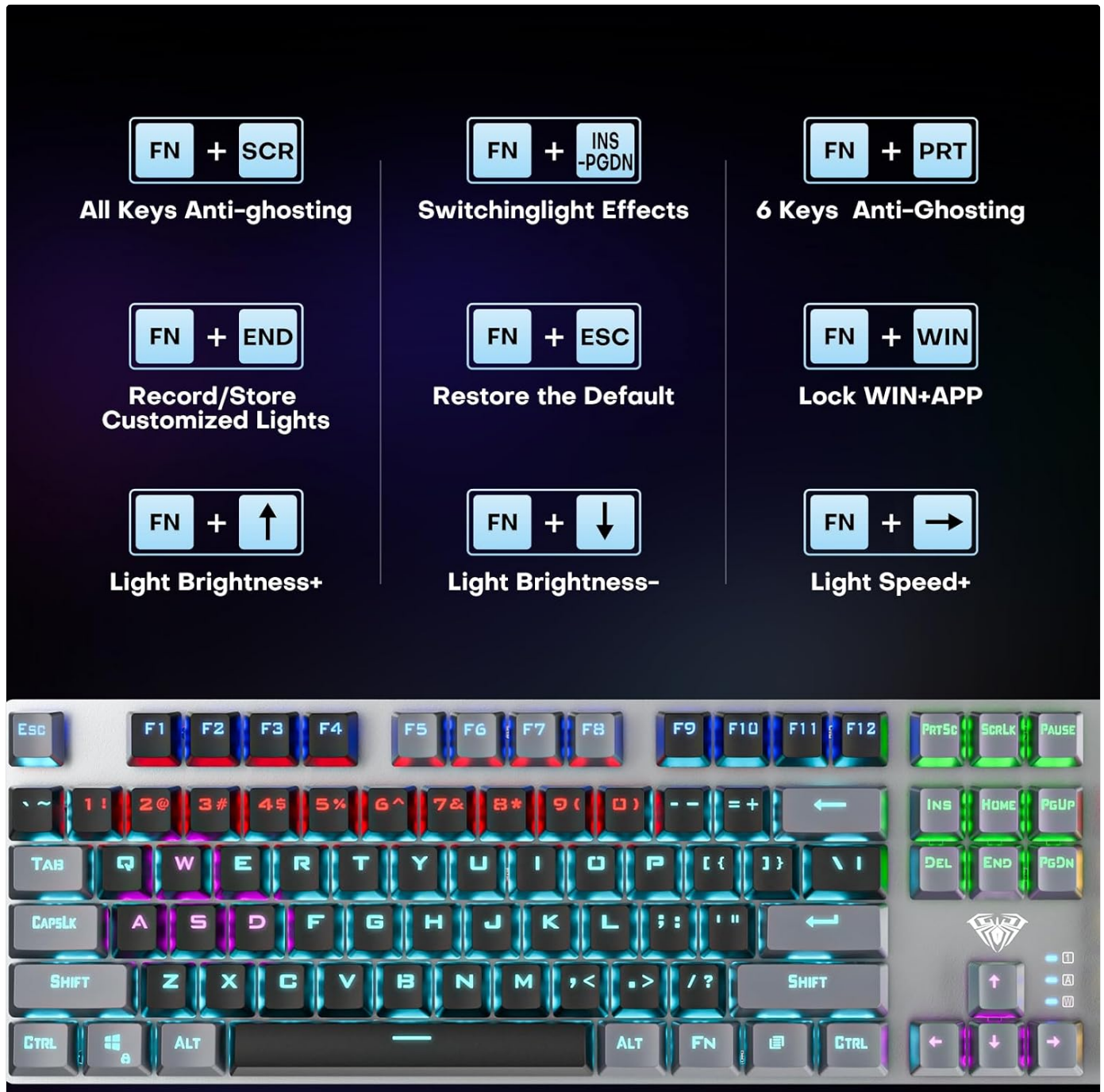
Image: Close-up of the AULA F2068Pro keyboard highlighting the FN key and its various combinations for controlling lighting effects and other functions.
