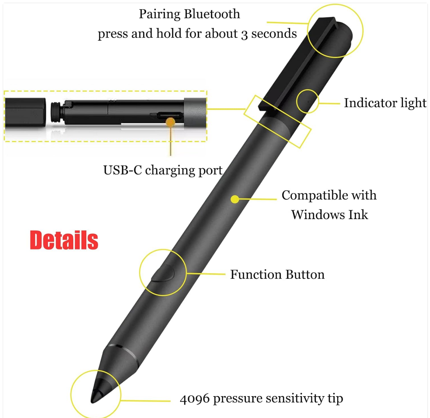
Figure 2: Mingxiong Tilt Pen Components
