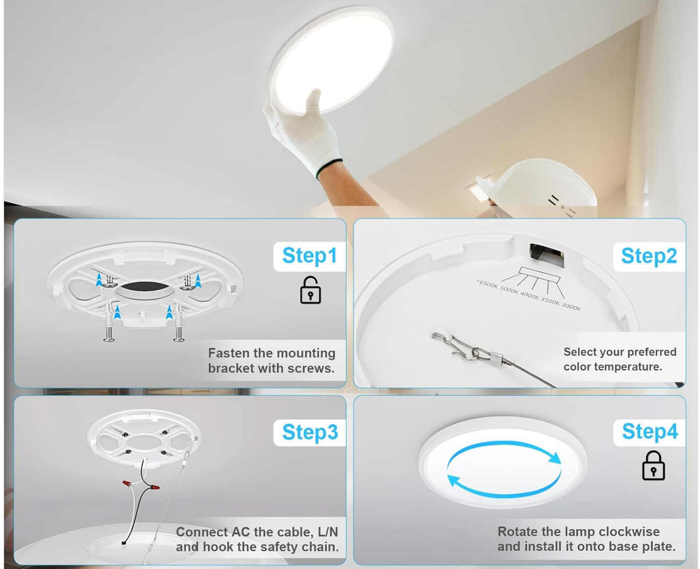
Image 4.1: Visual guide for the four-step installation process, from securing the bracket to final lamp attachment.
