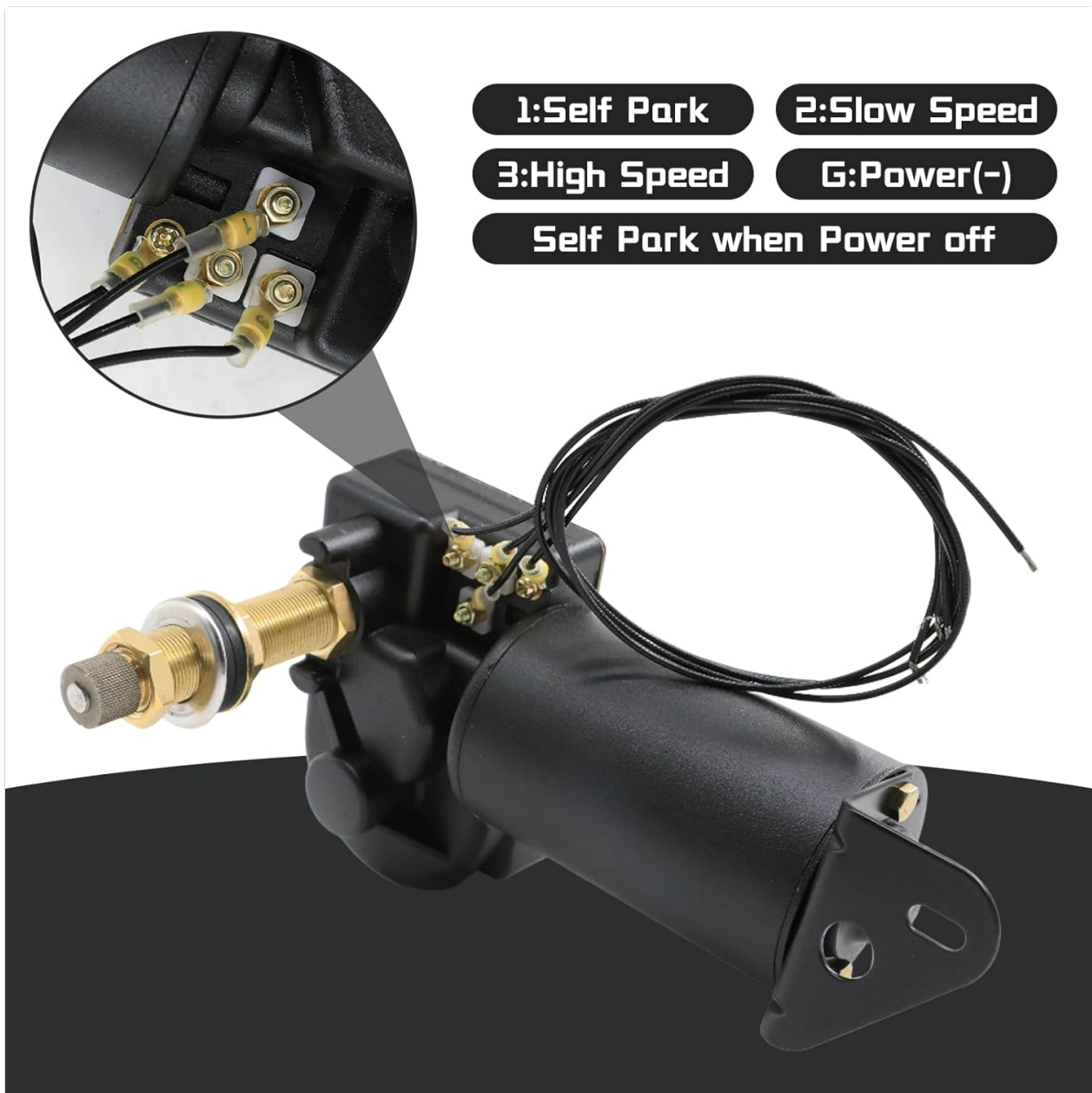
Figure 2: Wiring connections for the YBLKY Wiper Motor. The image shows four labeled terminals: 1: Self Park , 2: Slow Speed , 3: High Speed , and G: Power (-) . The 'Self Park' function activates when power is off.
