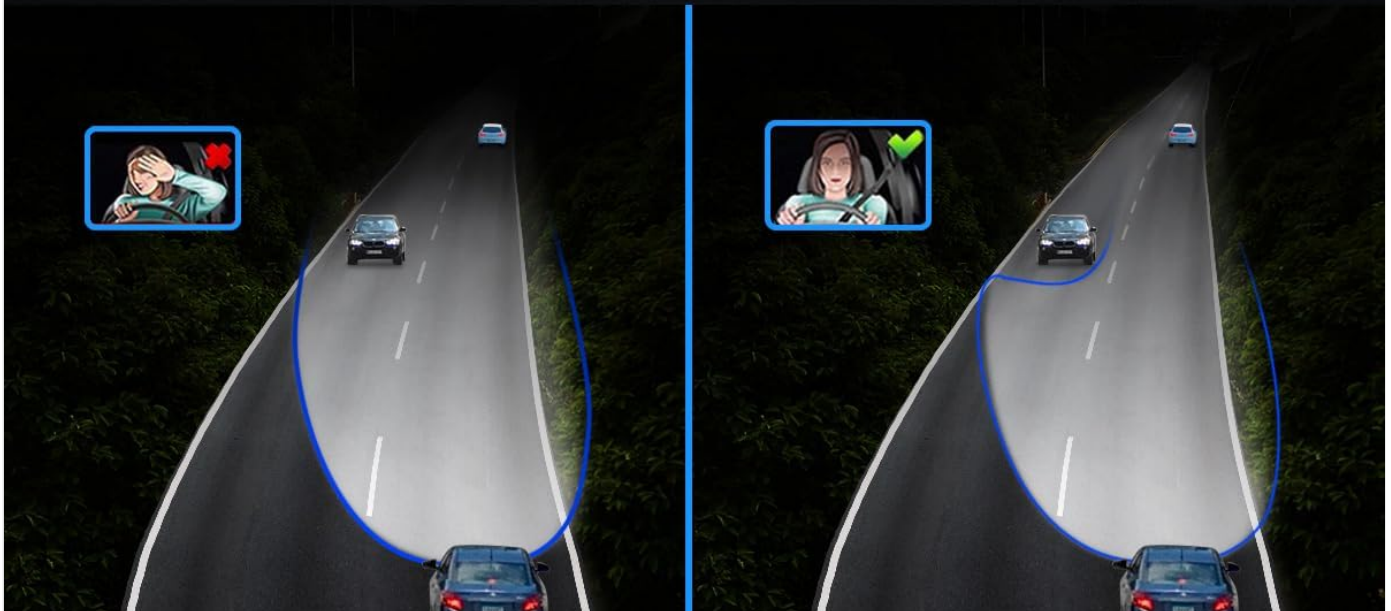
Image: Visual comparison demonstrating the improved light distribution and brightness provided by the reflective bowl design, showing a wider and more intense beam pattern.
