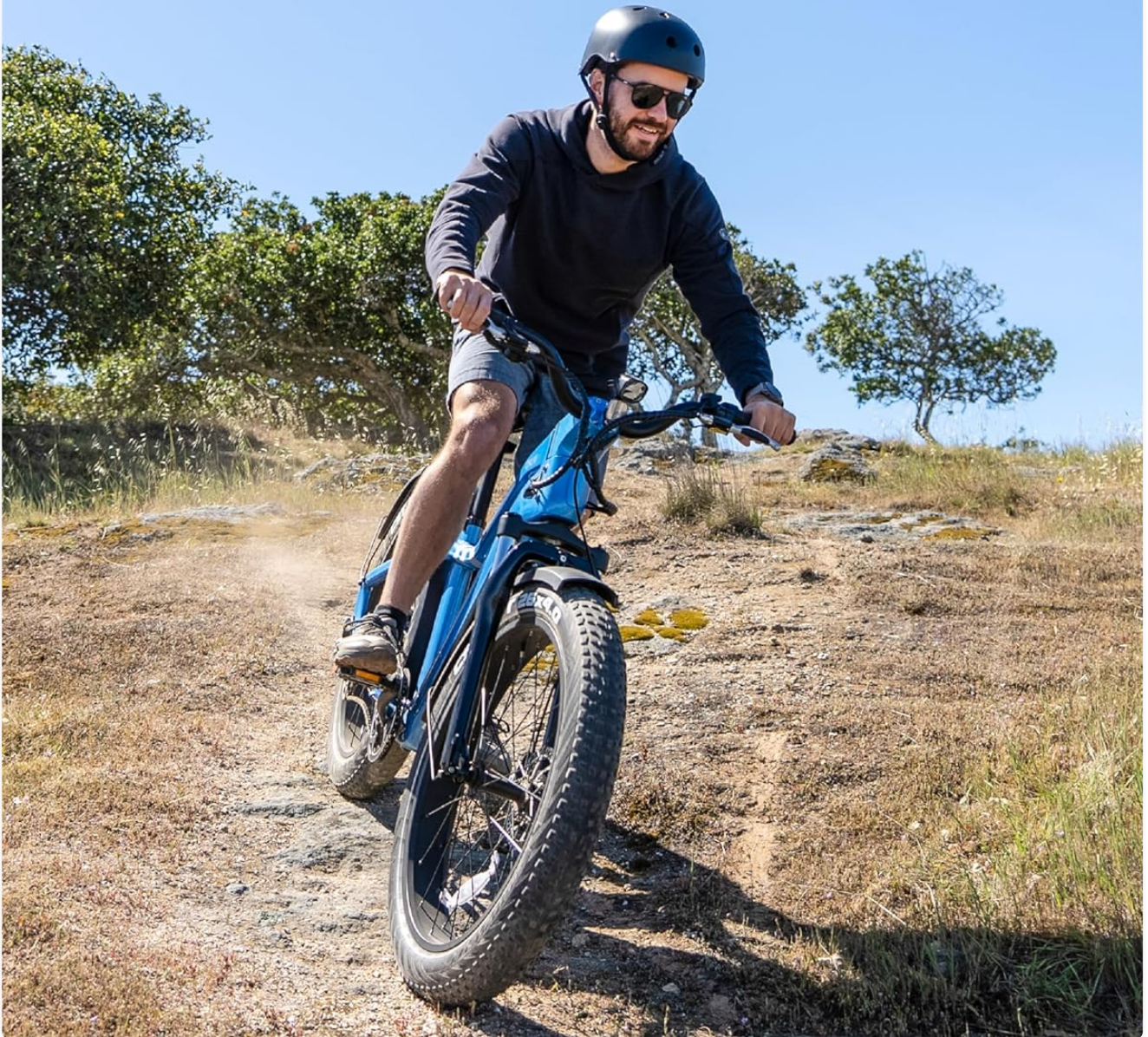
Figure 2.3: The fat tires and suspension allow for all-season, all-terrain use.
