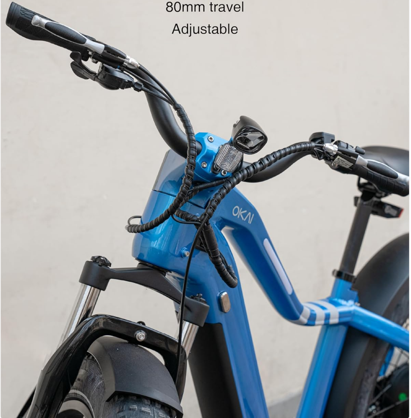
Figure 3.1: The hydraulic suspension fork provides 80mm of travel and includes a lockout feature.
