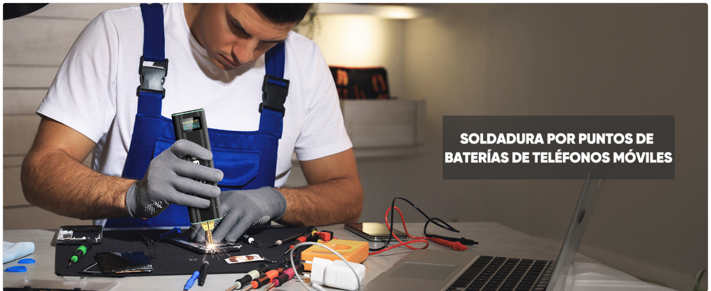
Image 6.3: A close-up of a technician performing spot welding on a mobile phone battery, highlighting the precision possible with the handheld device.
