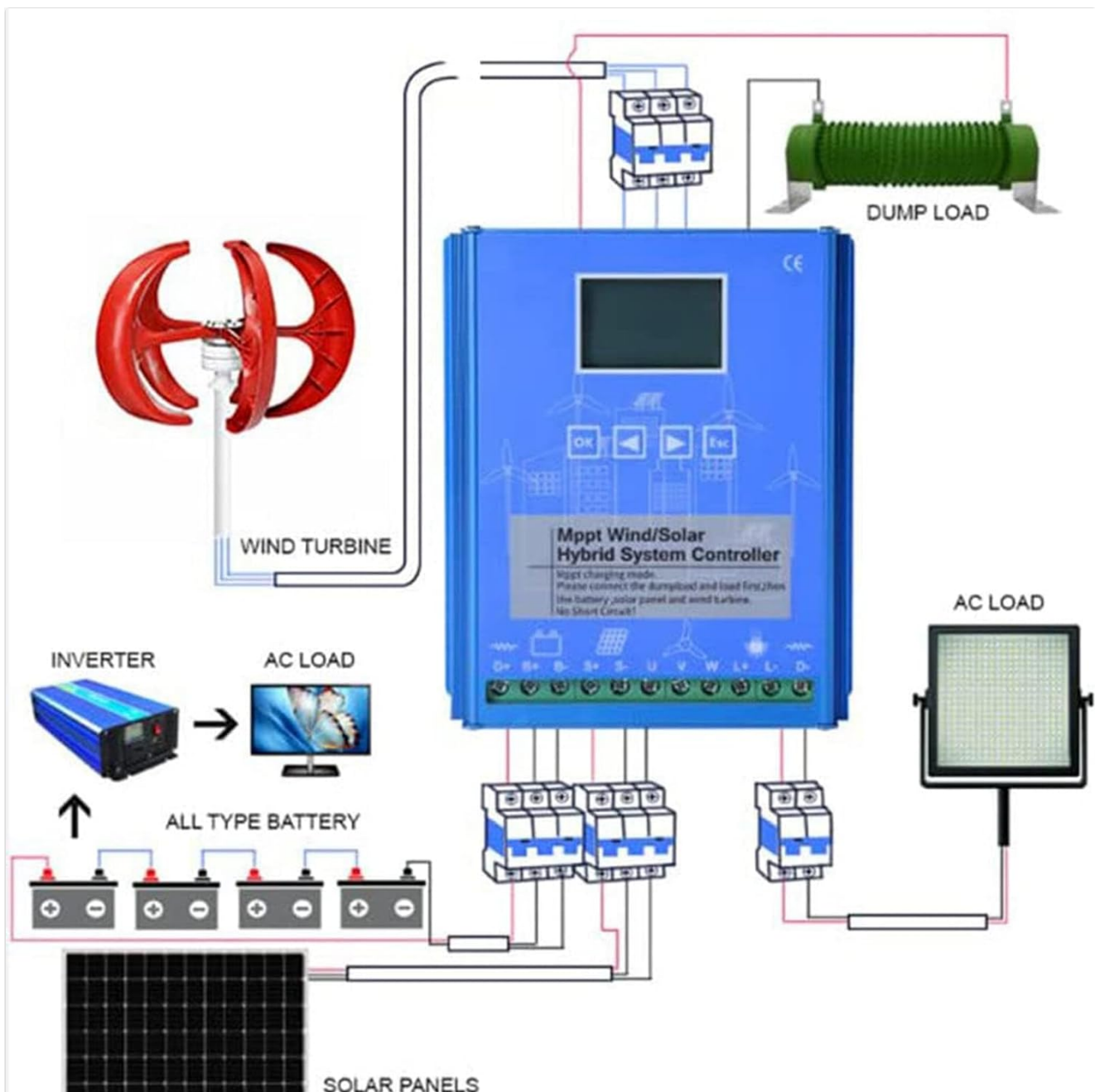
Figure 5.1: System wiring diagram. Ensure all connections are secure and correct polarity is observed.
