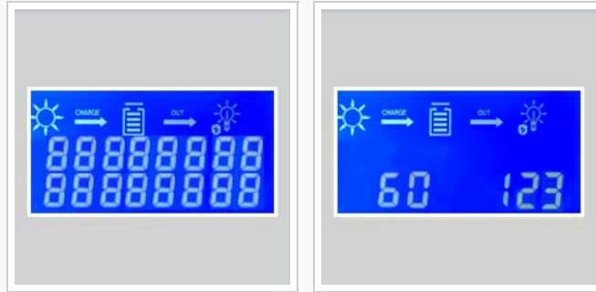
Figure 4: Example LCD screens. These images show various display modes, including icons for solar input, charging status, battery, load output, and numerical values for current and voltage.
