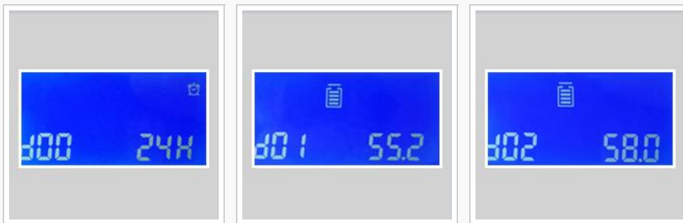
Figure 6: Battery Parameter Settings. These images show LCD screens for adjusting battery-related parameters such as battery type ('b00'), overcharge voltage ('b01'), and charge recovery voltage ('b02').
