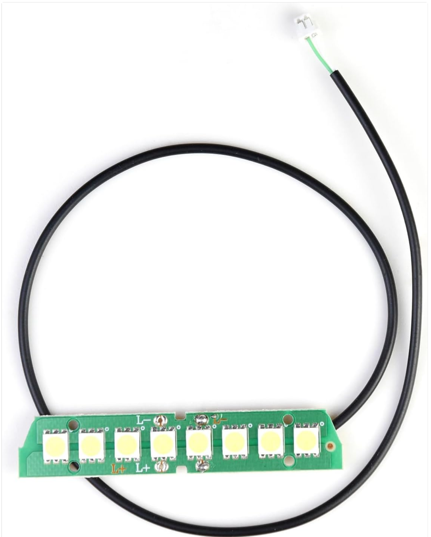
Figure 2.1: Front view of the X17-DJ03 LED Wire, showing the LED array and connector.
