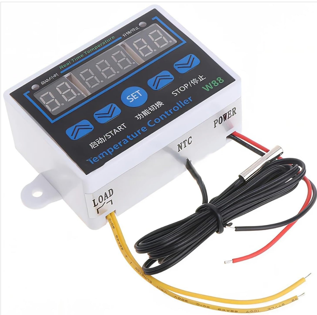
Figure 2.1: Side view of the XH-W1411 controller, showing the attached NTC temperature sensor and power/load wires.
