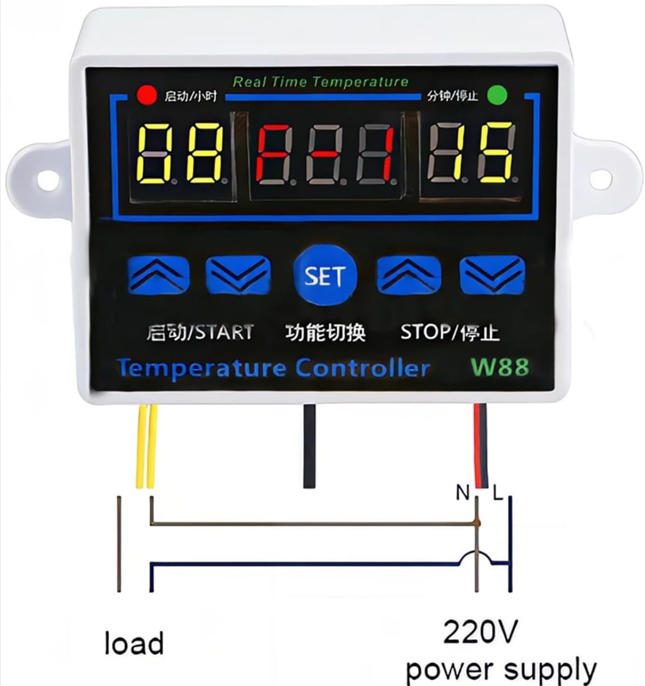
Figure 4.1: Wiring diagram for the AC 220V XH-W1411 controller. This diagram illustrates how to connect the 220V power supply and the load device to the controller's terminals.
