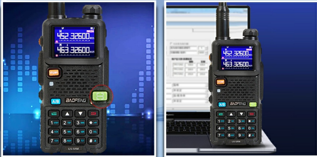
Image: The UV-5RM radio illustrating its one-click frequency copy function and PC manual programming capability.
