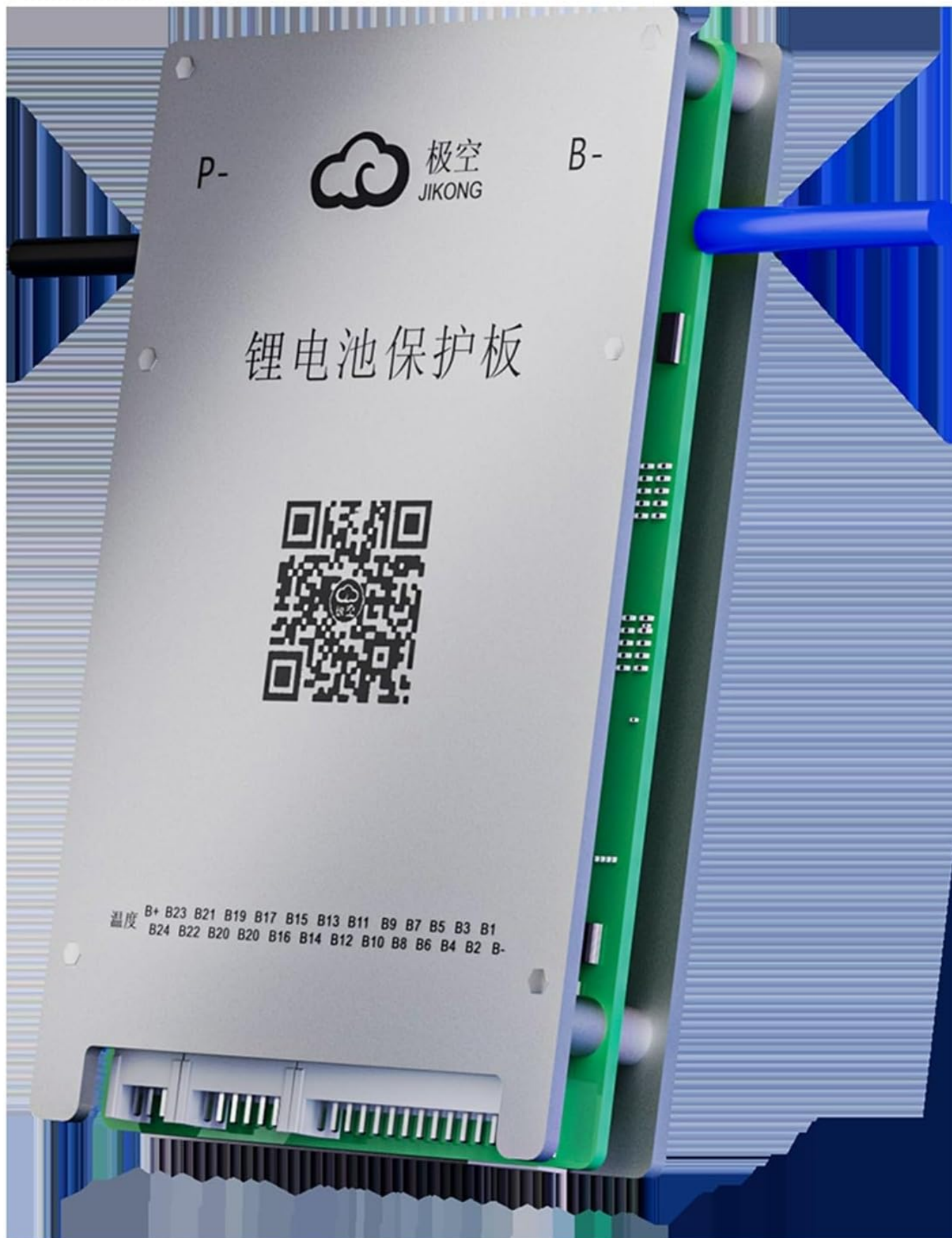
Image: Another view of the JK Smart BMS board, highlighting its robust construction and various connection points. For APP download and further information, scan the QR code or visit: http://qr17.cn/BApbC0
