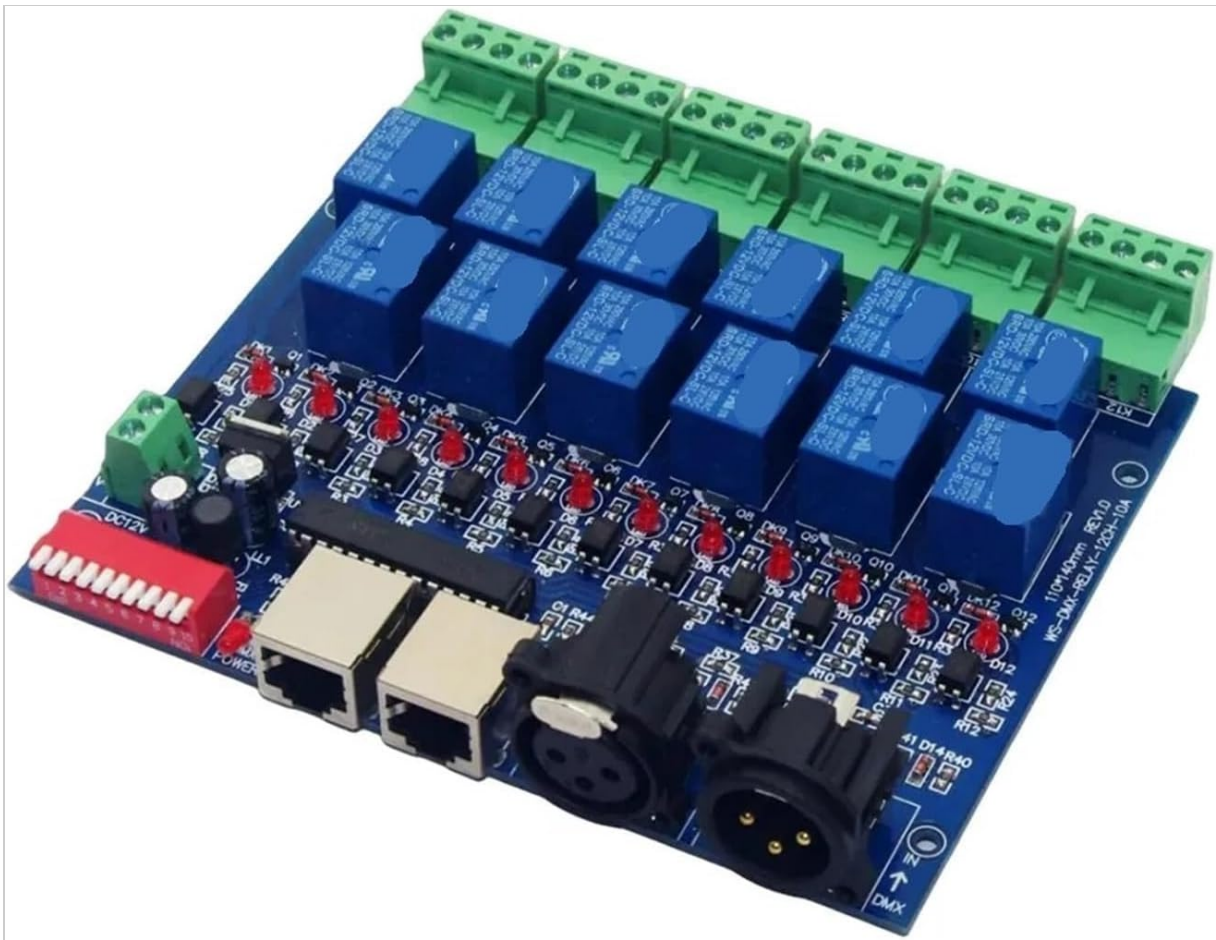
Figure 1: YIOGEQKWG WS-DMX-RELAY-12CH-10A DMX512 12-Channel Relay Switch Controller. This image displays the blue circuit board with twelve blue relays, green screw terminal blocks for power and relay outputs, two Ethernet ports, two DMX XLR ports, and a red DIP switch block for address setting. The board dimensions and model number are visible on the PCB.
