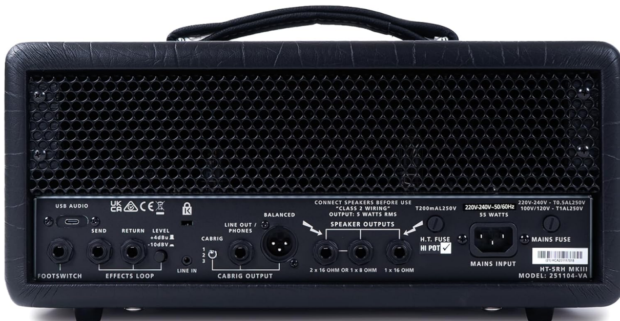
Image: Rear panel of the Blackstar HT-5RH MK III amplifier head, highlighting the speaker output jacks.
