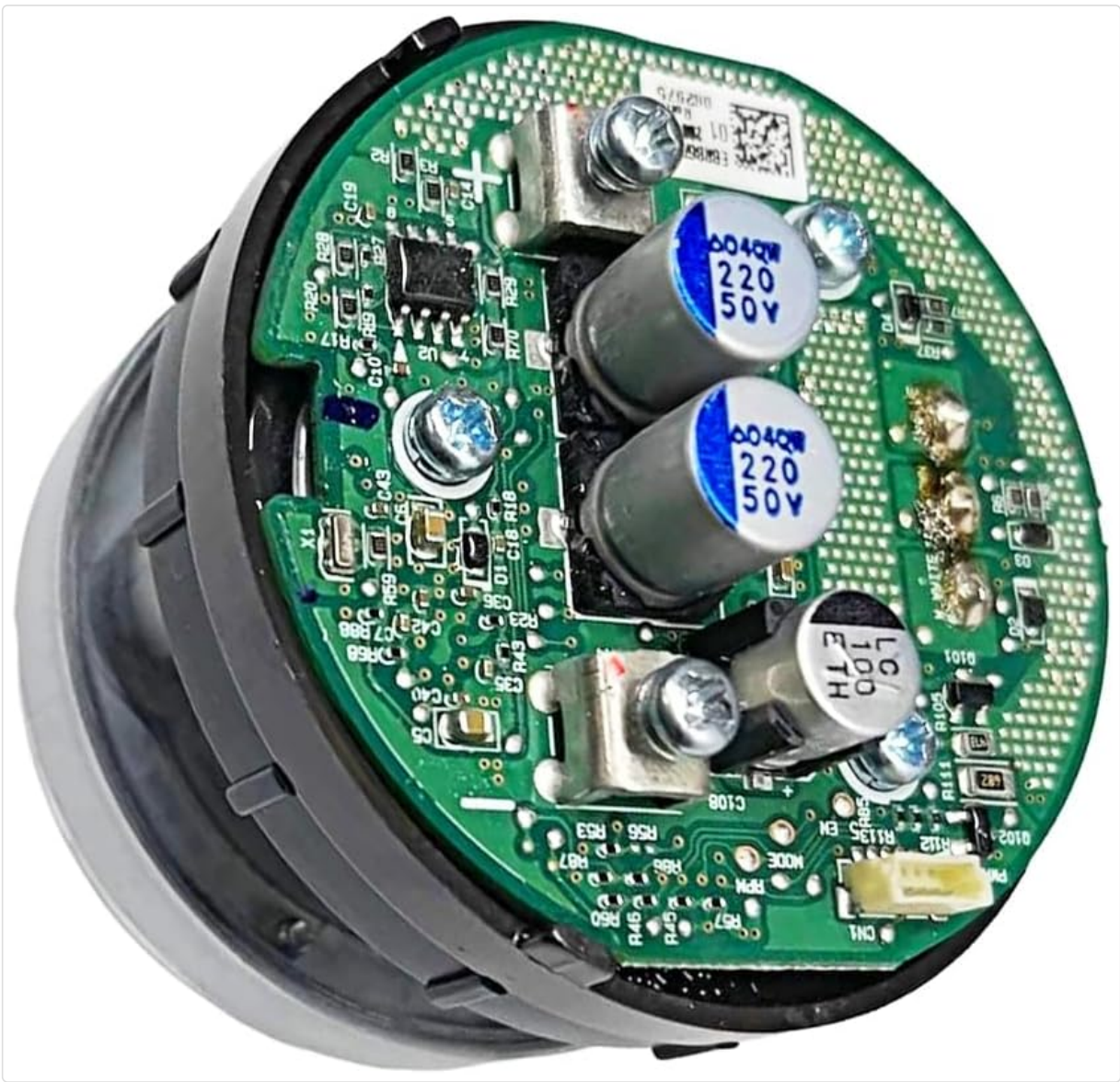
Image 2: Bottom view of the Goodsby Replacement Motor Unit, revealing the green circuit board with various electronic components, capacitors, and connection points. This side connects to the vacuum's internal wiring.
