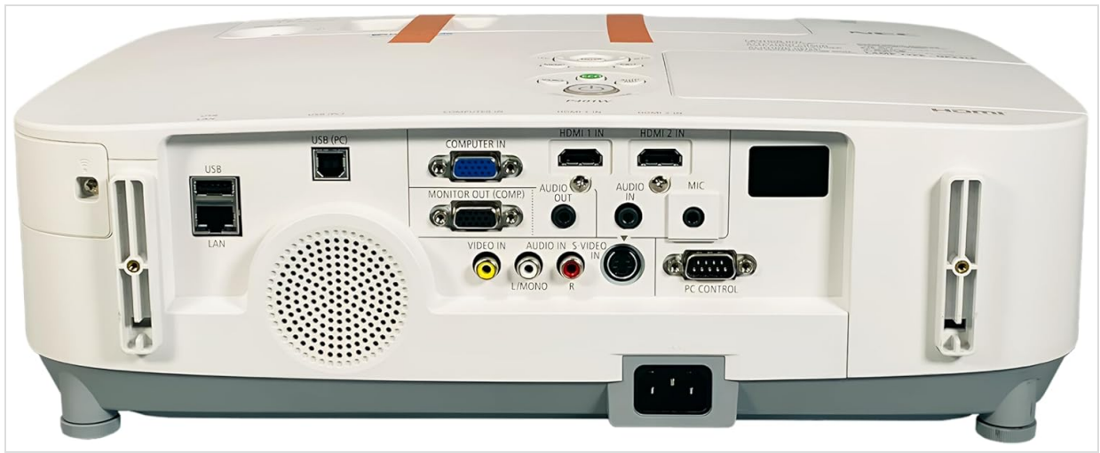
Image: Rear panel of the projector, displaying various ports including HDMI, USB, LAN, Computer In/Out (VGA), Video In (RCA), S-Video, Audio In/Out, and RS232 for control.
