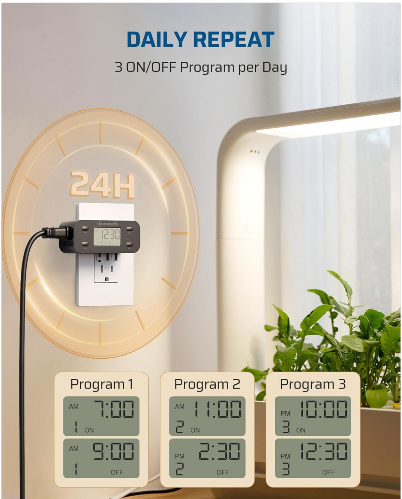
Figure 5: The timer supports up to three daily ON/OFF programs.
